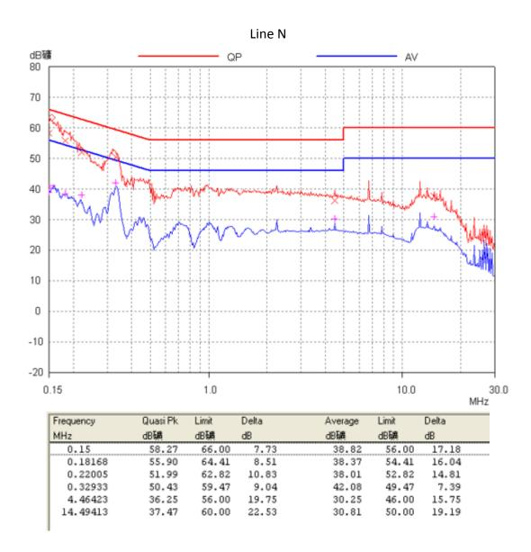
Remark: 1. Correct Factor = LISN Factor + Cable Loss, the value was added to Original Receiver Reading by the software automatically.
