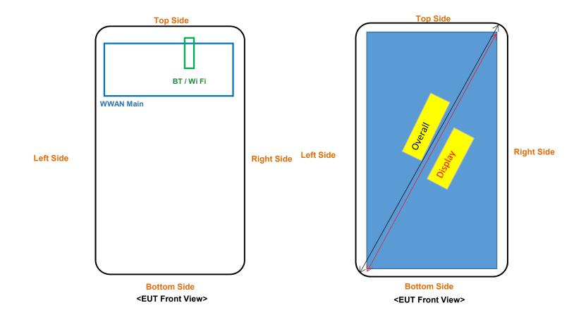
The separation distance for antenna to edge:
