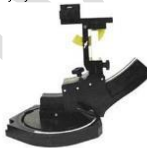
Device holder supplied by SPEAG
