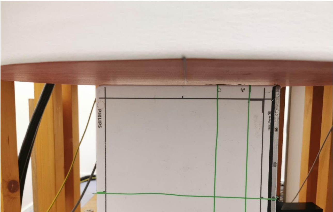
Figure 5. Left side of the DUT, 5mm separation distance
