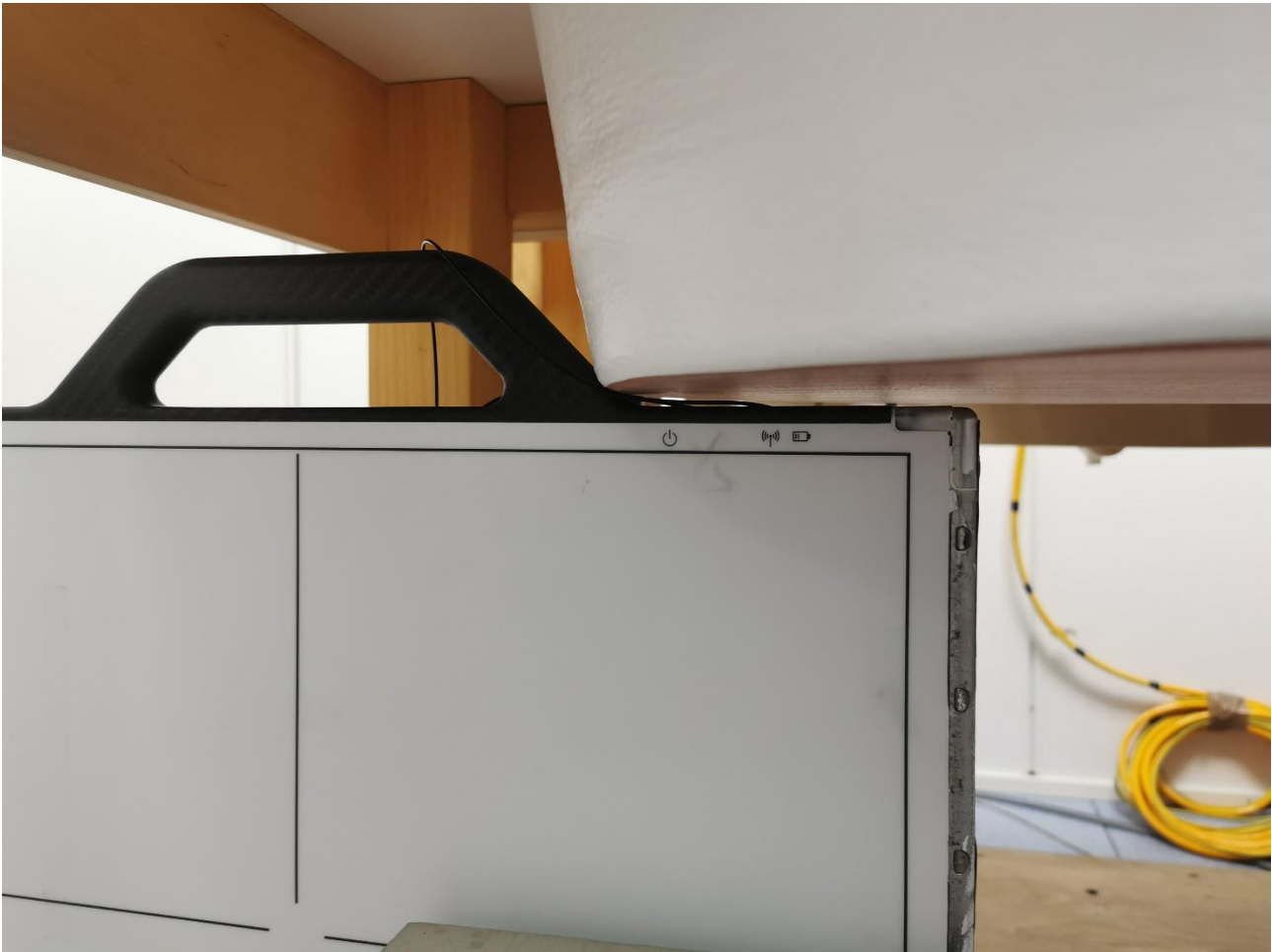
Figure 10. Left side of the DUT (3543EZh), 5mm separation distance
