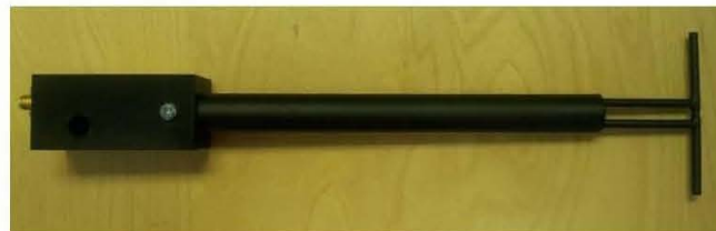
Figure 1 – MVG COMOSAR Validation Dipole
