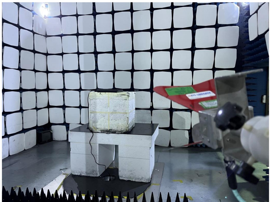
Radiation Emission Test Setup (1GHz to 18GHz)
