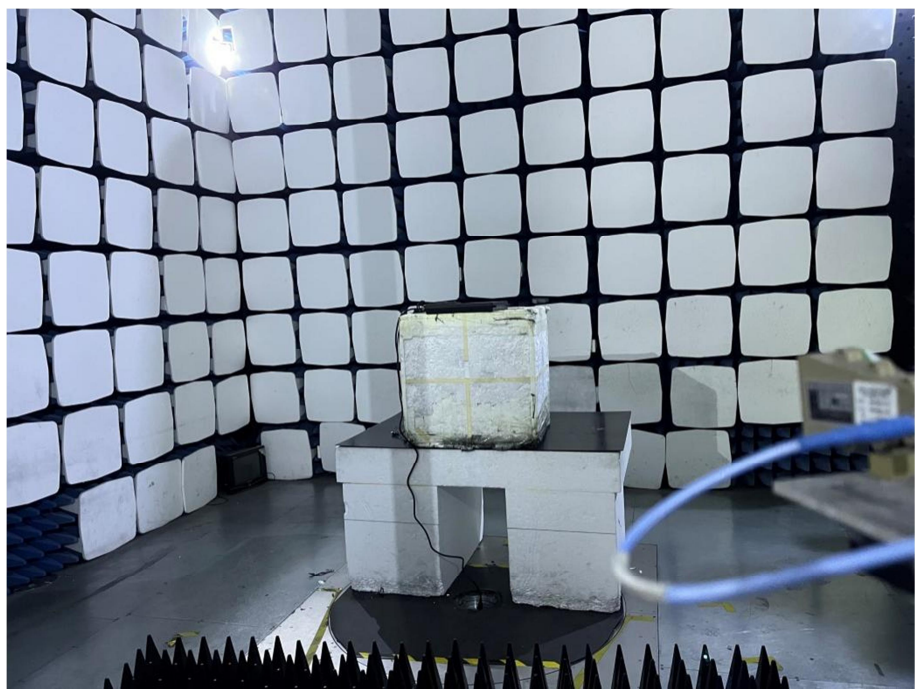
Radiation Emission Test Setup (Above 18GHz)
