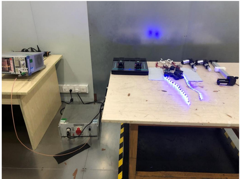
Conducted Emission Test Setup
