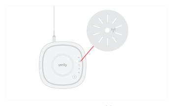
The light next to the connection symbol (1) will flash while establishing a connection. The Study Hub is ready to sync when the light changes to solid white, meaning a good connection has been made. The connection process may take up to 10 minutes depending on the connection quality.
