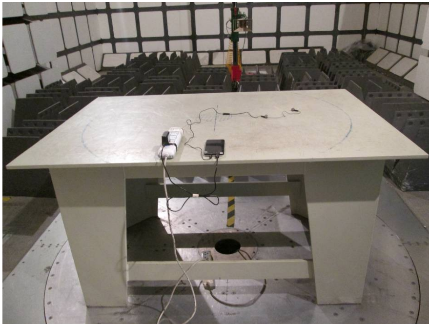
Radiated Emissions – Rear View (1-25 GHz)
