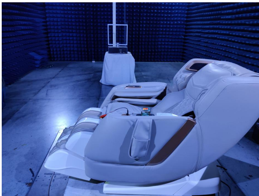
Photo of Radiated Emission Measurement Below 30MHz
