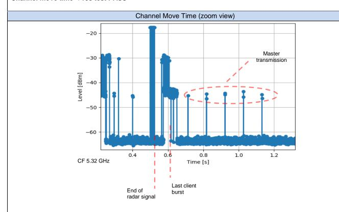
This zoom picture is generated with proprietary tool which process of the spectrum analyzer trace.
