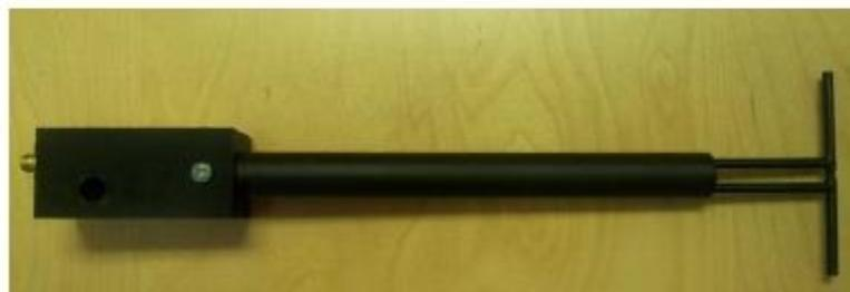
**Figure 1 – MVG COMOSAR Validation Dipole**
