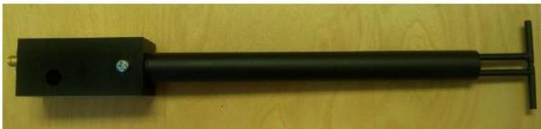
Figure 1 – MVG COMOSAR Validation Dipole
