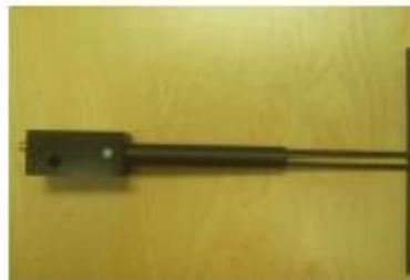
Figure 1 – MVG COMOSAR Validation Dipole
