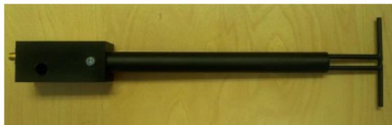
**Figure 1 – MVG COMOSAR Validation Dipole**
