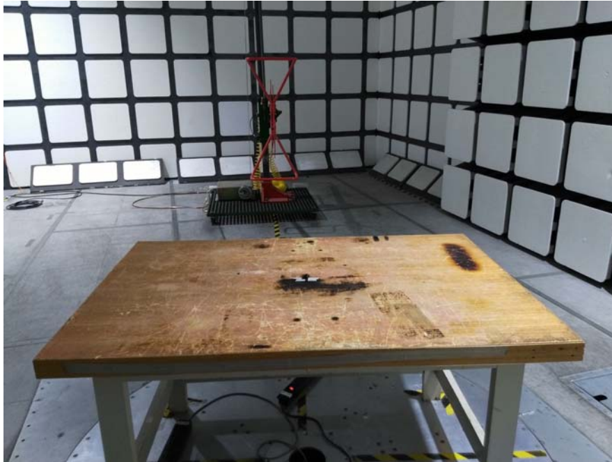
Radiated Emissions View (Below 1 GHz)
