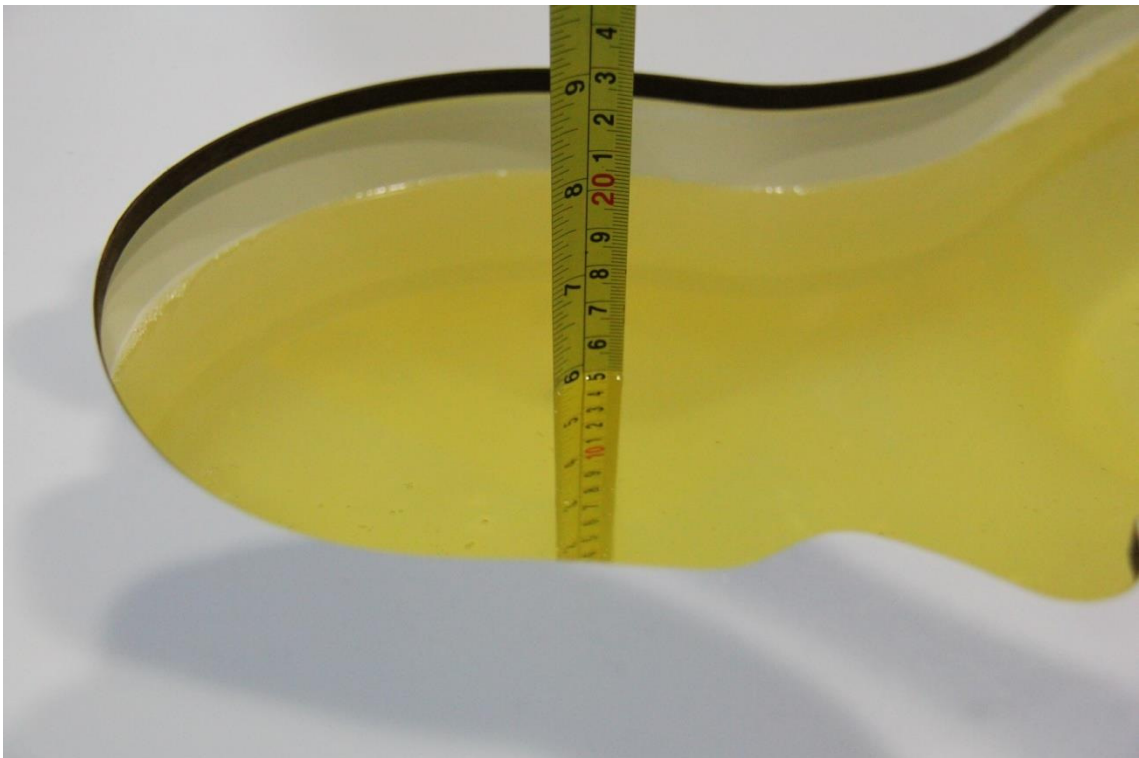
Picture 7-9: Liquid depth in the Head Phantom(2450MHz)
