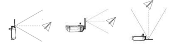
The optimal transmission range is where the antennas are facing toward the aircraft and the angle between the antennas and the back of the remote controller is  $180^{\circ}$  or  $270^{\circ}$ .
