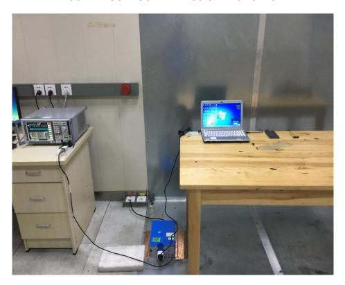
FCC RADIATED EMISSION TEST SETUP
