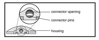
Look inside the connector opening of the transmitter to make sure that the connector pins are not damaged or corroded. If the connector pins are damaged or corroded, the transmitter cannot communicate with the charger or the app on your compatible mobile device. Contact the 24 Hour HelpLine. It may be time to replace your transmitter.
