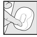
The tester can be used for one year. If you continue to use the tester for more than one year, the connector pins inside the transmitter could be damaged, because the tester cannot continue to provide a waterproof seal. For instructions on how to check the connector pins, see *Inspecting the transmitter connector pins, on page 8*.
