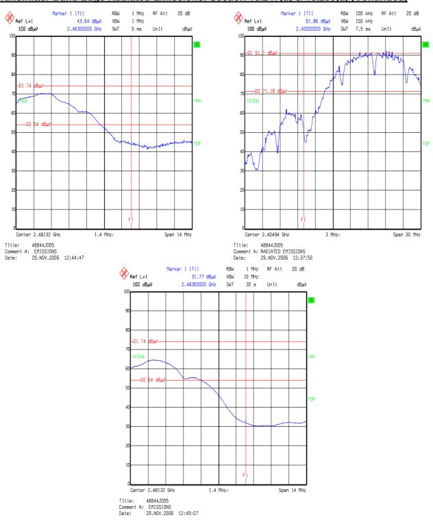
Note: The Band Edge plot at 2.4835 GHz shows a channel side band, not the transmit channel itself, thus the shape.
