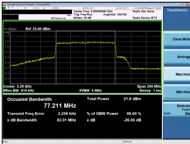
Plot 7-36. 26dB BW & 99% OBW Antenna WF5T (80MHz BW 802.11ax(SU) – Ch. 58, MCS4)
