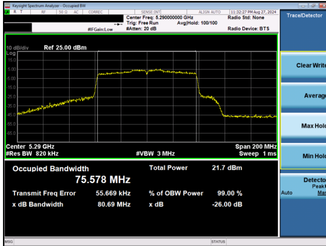
Plot 7-35. 26dB BW & 99% OBW Antenna WF5T (80MHz BW 802.11ac – Ch. 58, MCS4)
