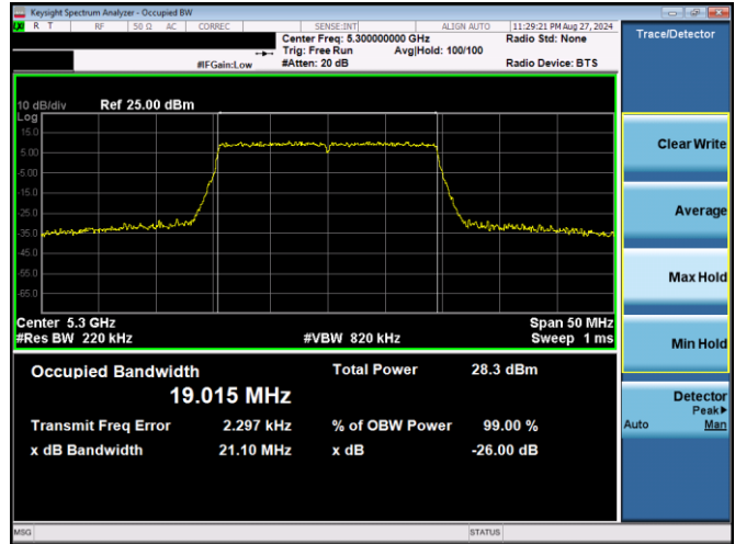
Plot 7-32. 26dB BW & 99% OBW Antenna WF5T (20MHz BW 802.11ax(SU) – Ch. 60, MCS4)
