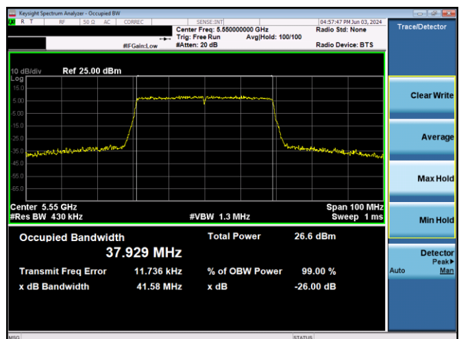
Plot 7-40. 26dB BW & 99% OBW Antenna WF5T (40MHz BW 802.11ax(SU) – Ch. 110, MCS4)
