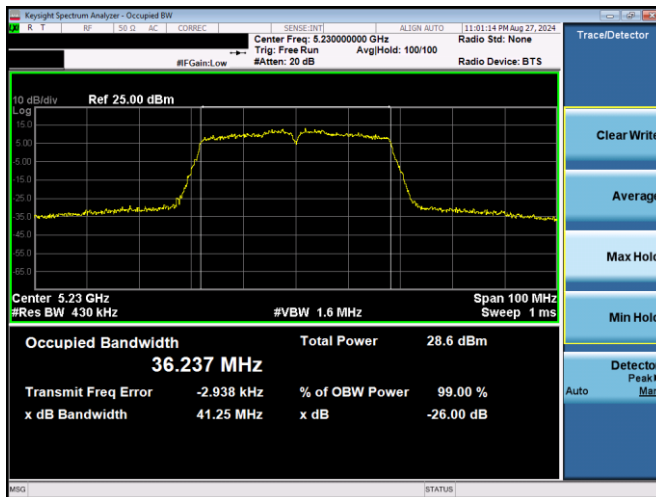
Plot 7-3. 26dB BW & 99% OBW Antenna WF5T (40MHz BW 802.11n – Ch. 46, MCS2)
