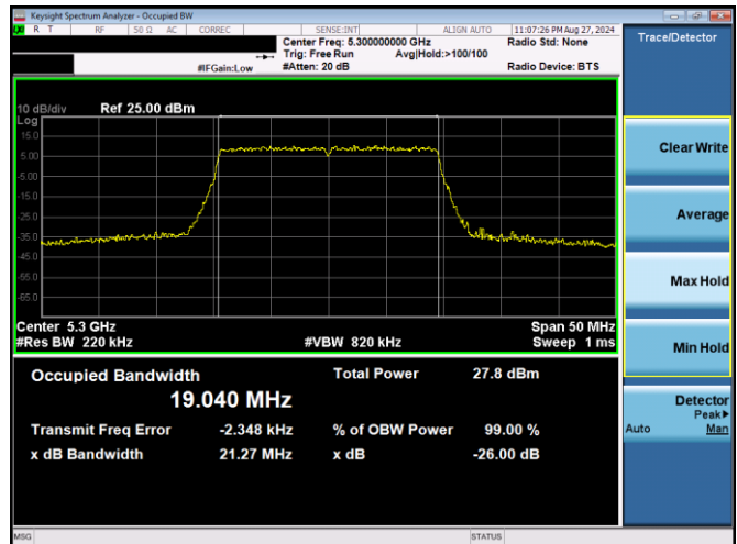
Plot 7-10. 26dB BW & 99% OBW Antenna WF5T (20MHz BW 802.11ax(SU) – Ch. 60, MCS2)
