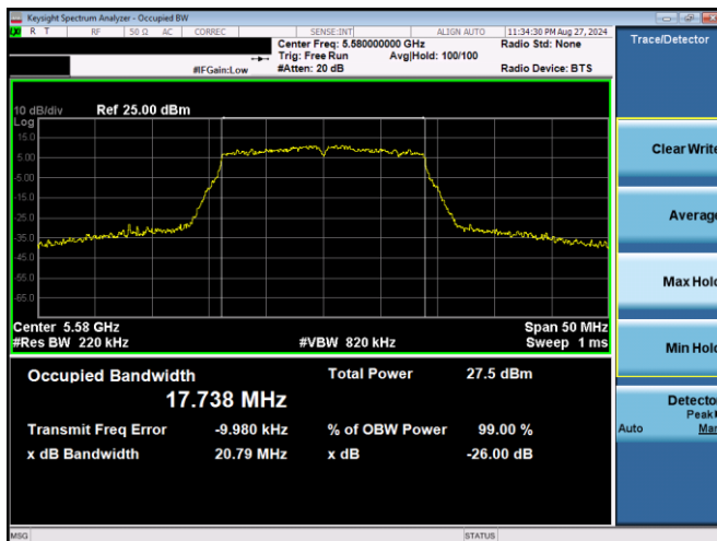
Plot 7-37. 26dB BW & 99% OBW Antenna WF5T (20MHz BW 802.11n – Ch. 116, MCS4)
