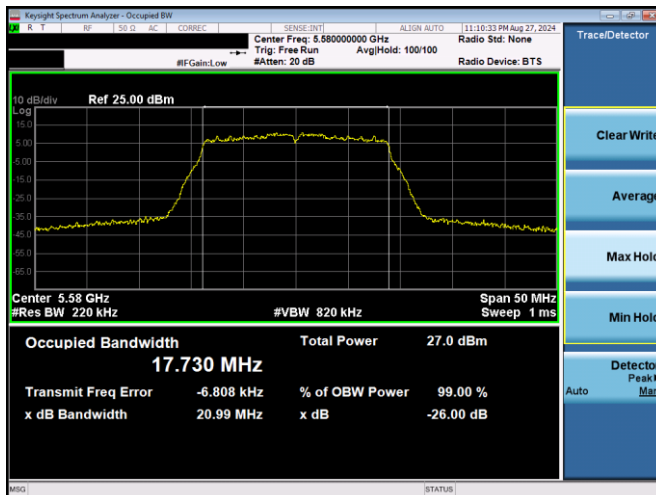
Plot 7-15. 26dB BW & 99% OBW Antenna WF5T (20MHz BW 802.11n – Ch. 116, MCS2)
