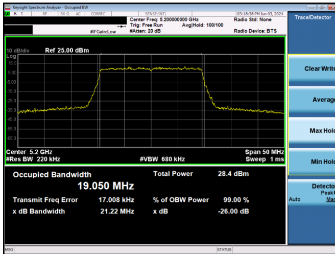
Plot 7-2. 26dB BW & 99% OBW Antenna WF5T (20MHz BW 802.11ax(SU) – Ch. 40, MCS2)
