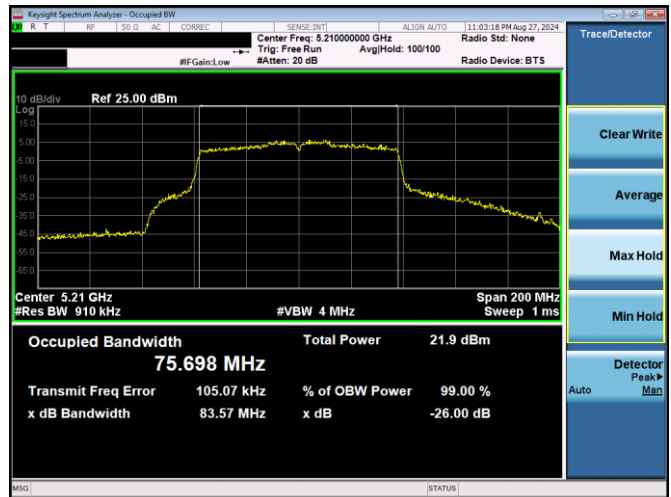
Plot 7-5. 26dB BW & 99% OBW Antenna WF5T (80MHz BW 802.11ac – Ch. 42, MCS2)
