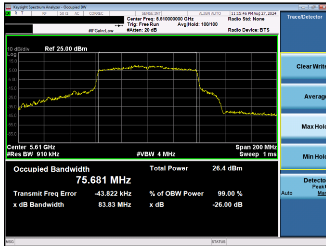
Plot 7-19. 26dB BW & 99% OBW Antenna WF5T (80MHz BW 802.11ac – Ch. 122, MCS2)
