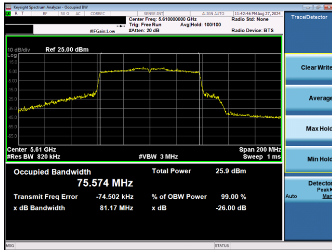
Plot 7-41. 26dB BW & 99% OBW Antenna WF5T (80MHz BW 802.11ac – Ch. 122, MCS4)
