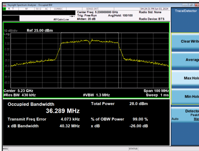
Plot 7-25. 26dB BW & 99% OBW Antenna WF5T (40MHz BW 802.11n – Ch. 46, MCS4)
