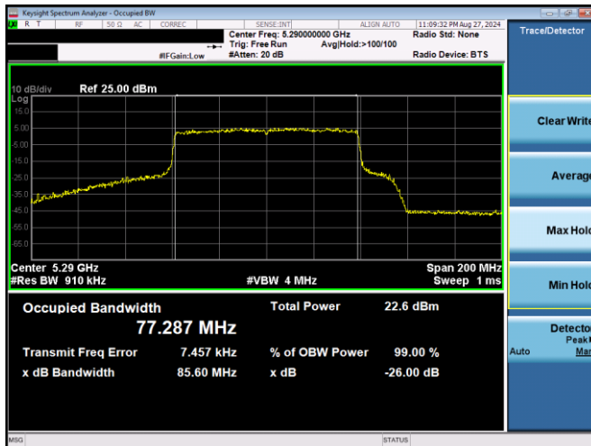
Plot 7-14. 26dB BW & 99% OBW Antenna WF5T (80MHz BW 802.11ax(SU) – Ch. 58, MCS2)
