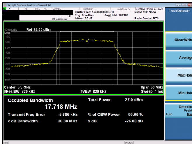
Plot 7-9. 26dB BW & 99% OBW Antenna WF5T (20MHz BW 802.11n – Ch. 60, MCS2)
