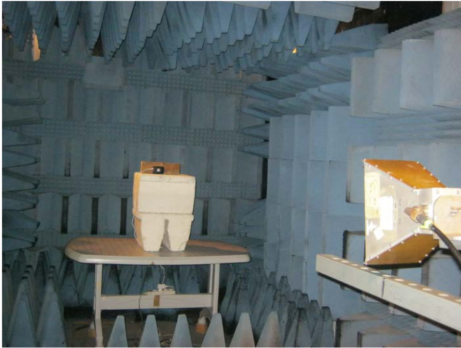
Figure 2. Intermodulated Radiated Emission Test
