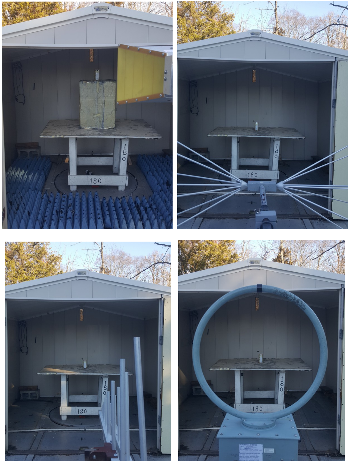
Figure 3.1 Radiated Test Setup
