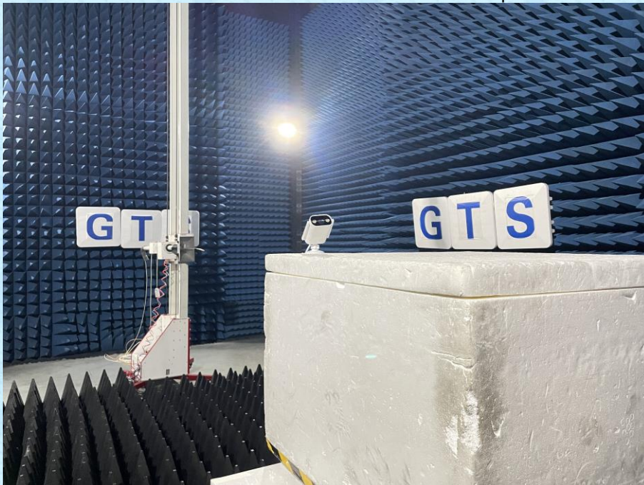
Radiated Emission Above 1GHz Test Setup
