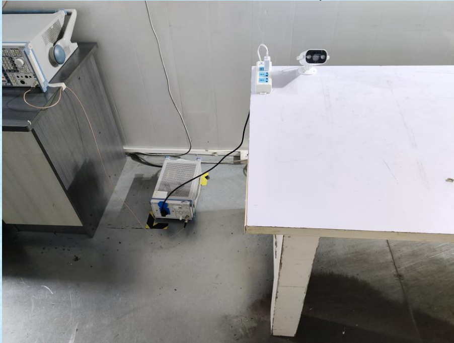
Conducted Emission Test Setup
