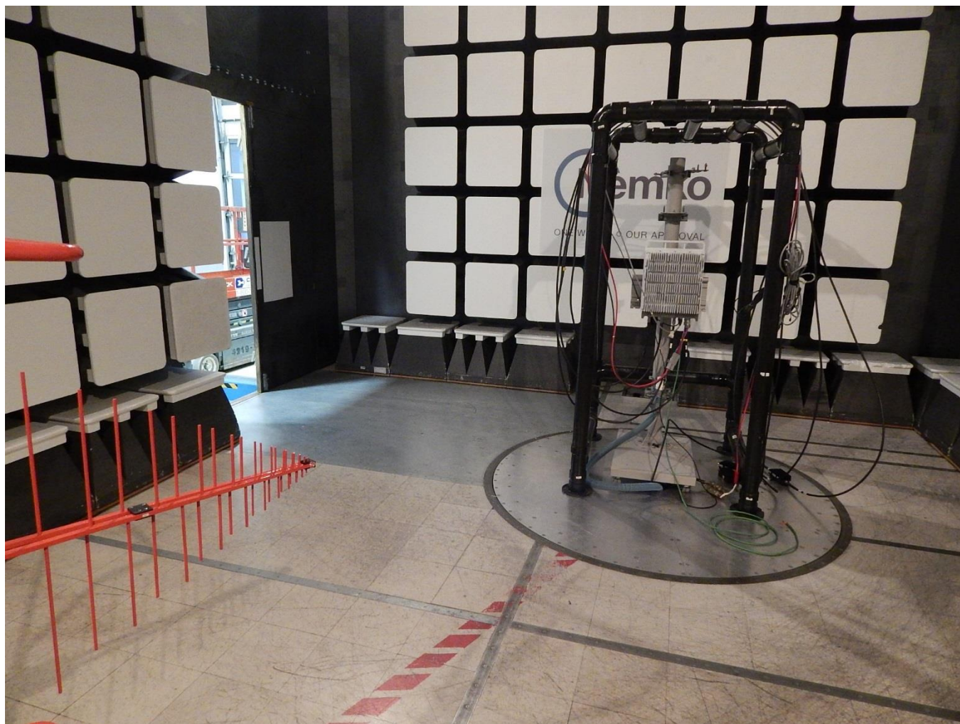
Figure 3.6-4: EUT Set-up for Radiated Compliance Testing
