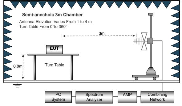
(C) Radiated Emission Test-Up Frequency Above 1GHz
