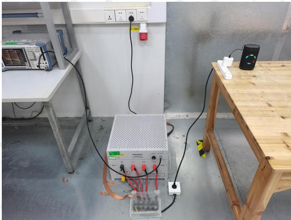
Photo of Conducted Emission Measurement
