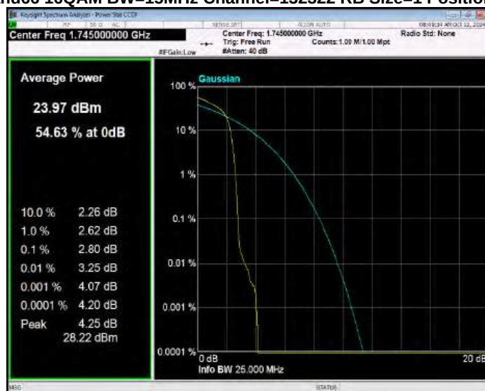
Band66 16QAM BW=15MHz Channel=132597 RB Size=1 Position=#0
