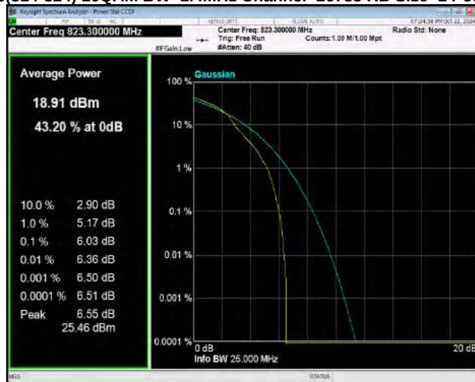
Band26(814-824) 16QAM BW=10MHz Channel=26740 RB Size=1 Position=#0
