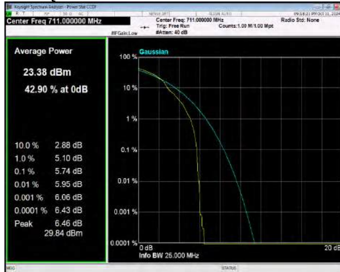
Band17 16QAM BW=5MHz Channel=23755 RB Size=1 Position=#0
