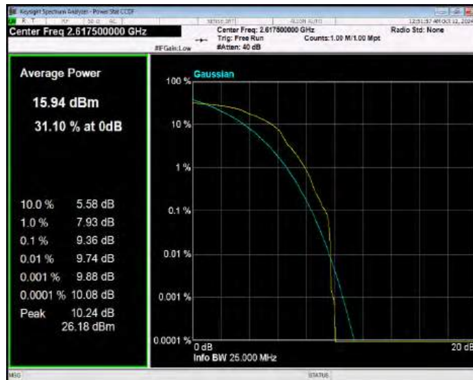
Band38 QPSK BW=10MHz Channel=37800 RB Size=1 Position=#0
