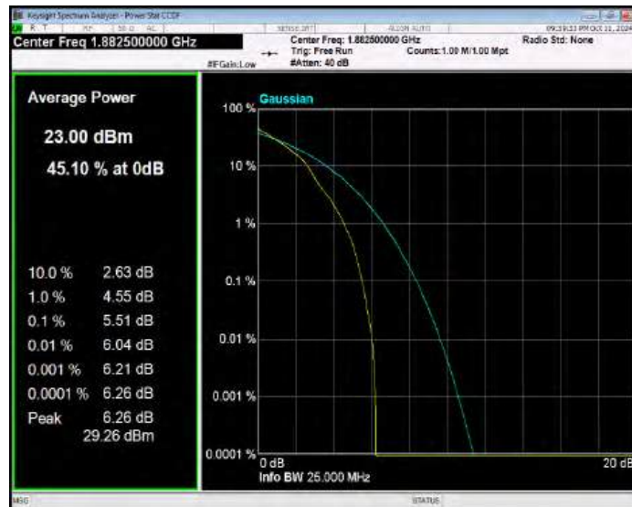
Band25 QPSK BW=10MHz Channel=26640 RB Size=1 Position=#0
