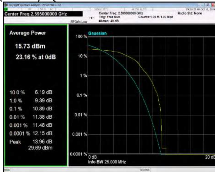
Band41(2535-2655) 16QAM BW=15MHz Channel=41165 RB Size=1 Position=#0
