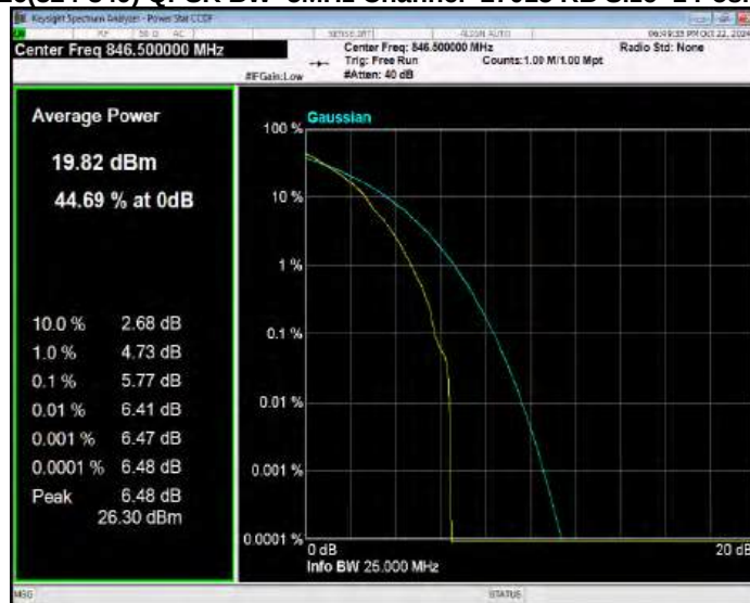
Band26(814-824) 16QAM BW=1.4MHz Channel=26697 RB Size=1 Position=#0
