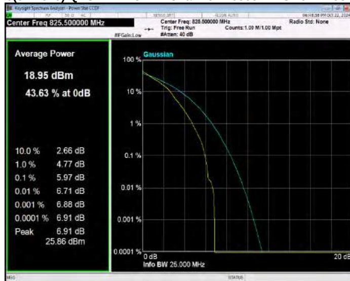
Band26(824-849) QPSK BW=3MHz Channel=26915 RB Size=1 Position=#0
