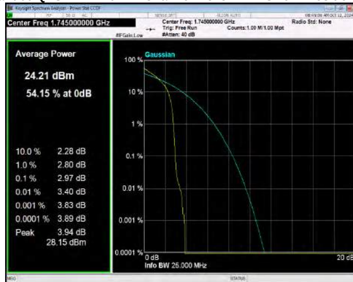
Band66 QPSK BW=10MHz Channel=132622 RB Size=1 Position=#0
