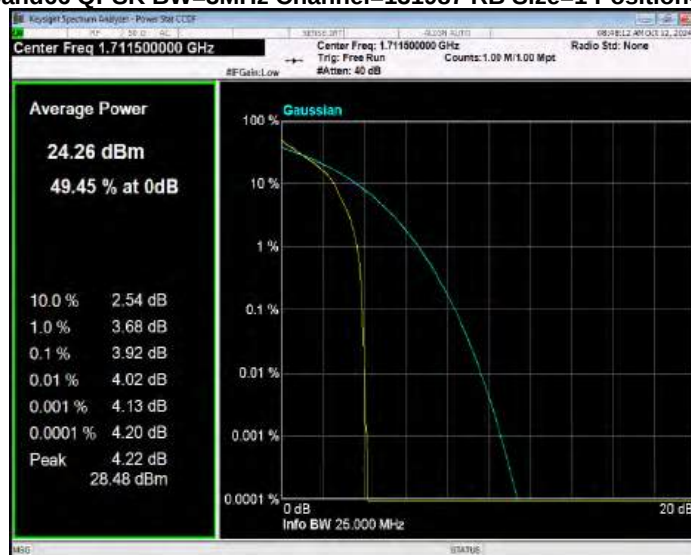
Band66 QPSK BW=3MHz Channel=132322 RB Size=1 Position=#0
