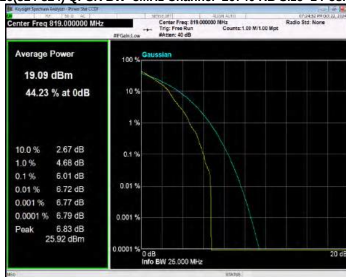
Band26(814-824) QPSK BW=3MHz Channel=26775 RB Size=1 Position=#0
