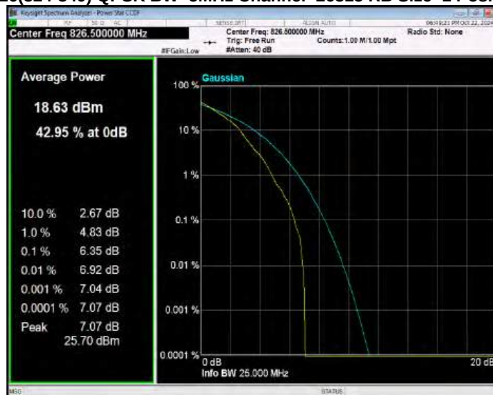
Band26(824-849) QPSK BW=5MHz Channel=26915 RB Size=1 Position=#0
