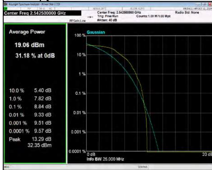
Band41(2535-2655) QPSK BW=15MHz Channel=40640 RB Size=1 Position=#0
