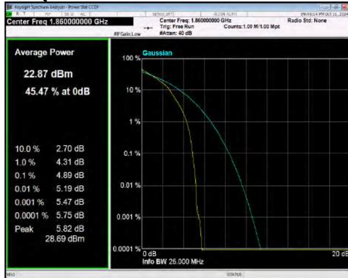
Band25 QPSK BW=20MHz Channel=26365 RB Size=1 Position=#0
