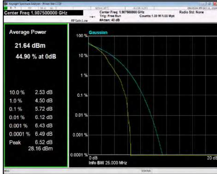
Band25 QPSK BW=20MHz Channel=26140 RB Size=1 Position=#0
