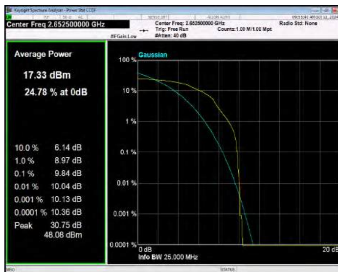
Band41(2535-2655) QPSK BW=10MHz Channel=40090 RB Size=1 Position=#0
