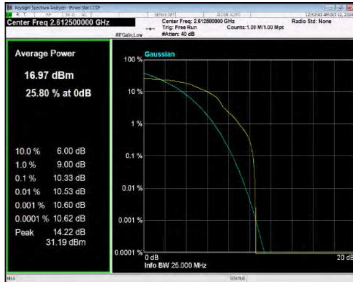
Band38 16QAM BW=20MHz Channel=37850 RB Size=1 Position=#0
