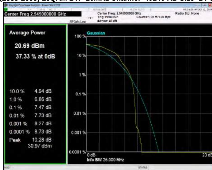
Band41(2535-2655) 16QAM BW=20MHz Channel=40640 RB Size=1 Position=#0
