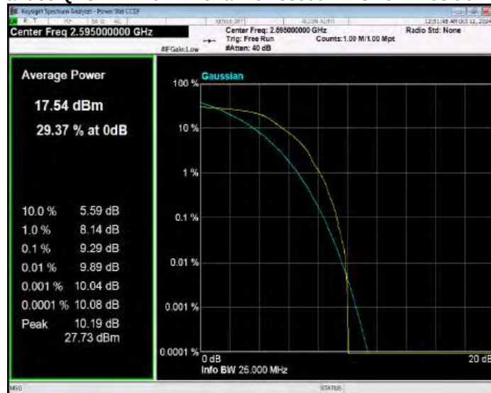
Band38 QPSK BW=5MHz Channel=38225 RB Size=1 Position=#0
