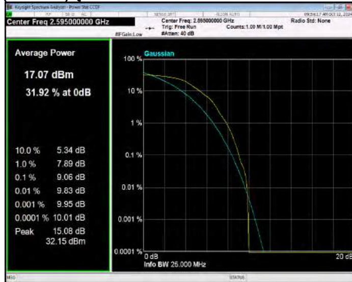
Band41(2535-2655) QPSK BW=15MHz Channel=41165 RB Size=1 Position=#0
