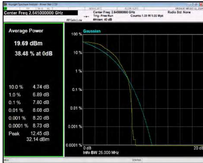
Band41(2535-2655) QPSK BW=5MHz Channel=40065 RB Size=1 Position=#0
