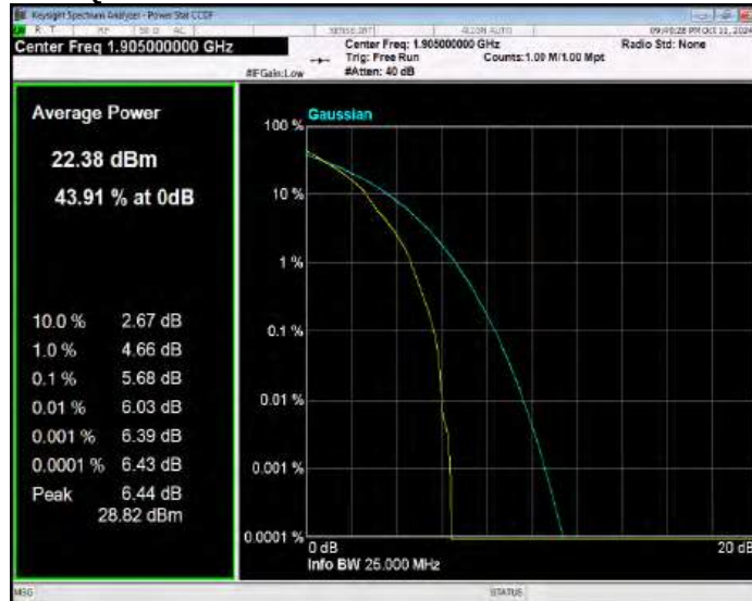
Band25 QPSK BW=3MHz Channel=26055 RB Size=1 Position=#0
