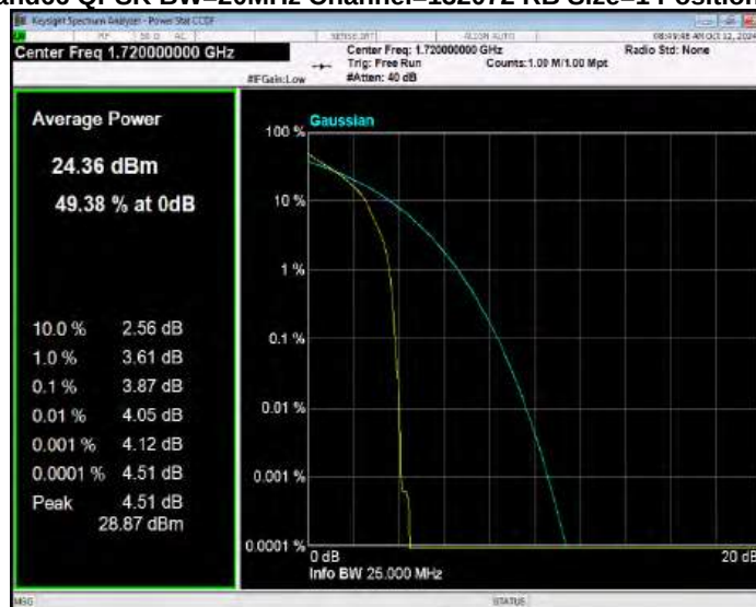
Band66 QPSK BW=20MHz Channel=132322 RB Size=1 Position=#0
