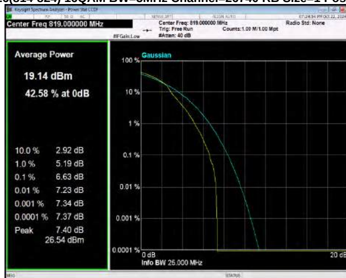
Band26(814-824) 16QAM BW=3MHz Channel=26775 RB Size=1 Position=#0
