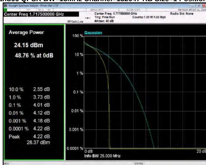
Band66 QPSK BW=15MHz Channel=132322 RB Size=1 Position=#0
