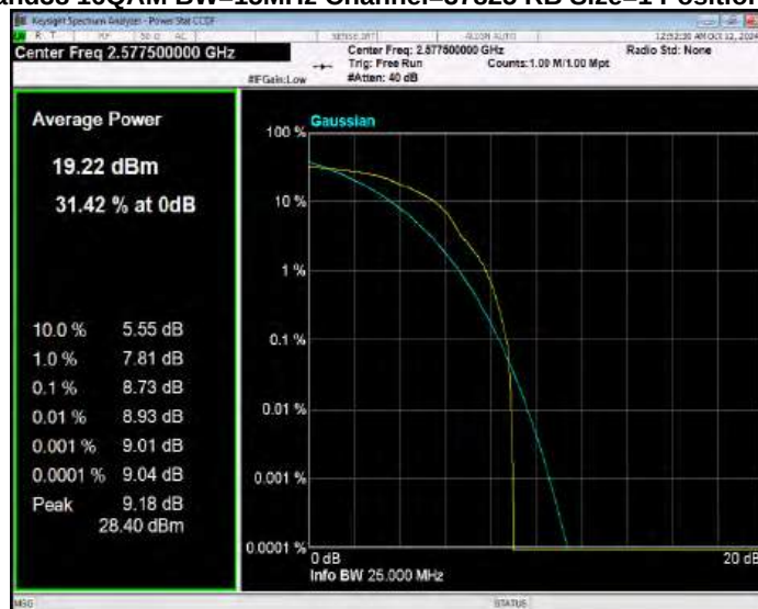
Band38 16QAM BW=15MHz Channel=38000 RB Size=1 Position=#0
