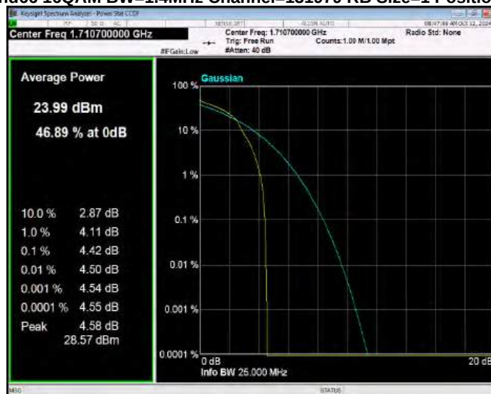
Band66 16QAM BW=1.4MHz Channel=132322 RB Size=1 Position=#0
