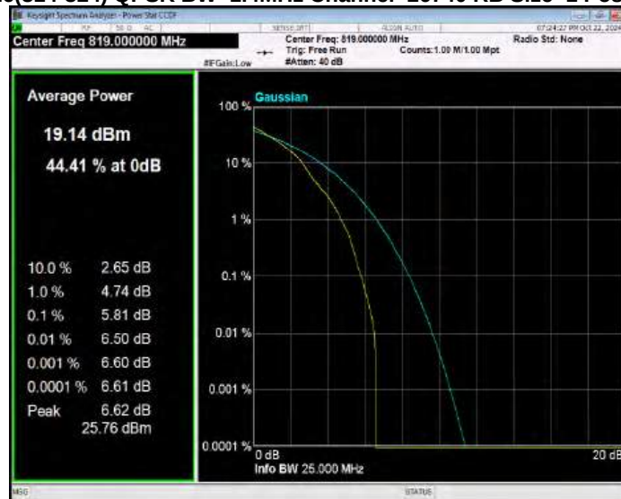
Band26(814-824) QPSK BW=1.4MHz Channel=26783 RB Size=1 Position=#0
