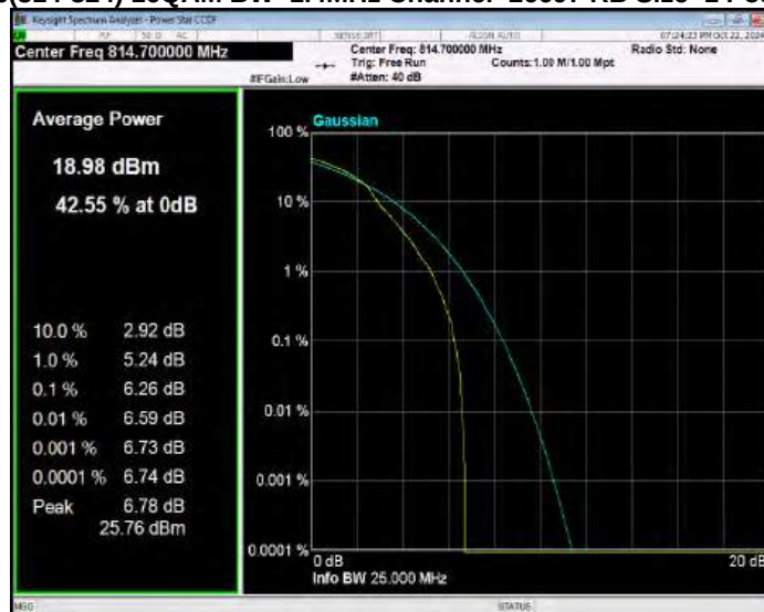
Band26(814-824) 16QAM BW=1.4MHz Channel=26740 RB Size=1 Position=#0
