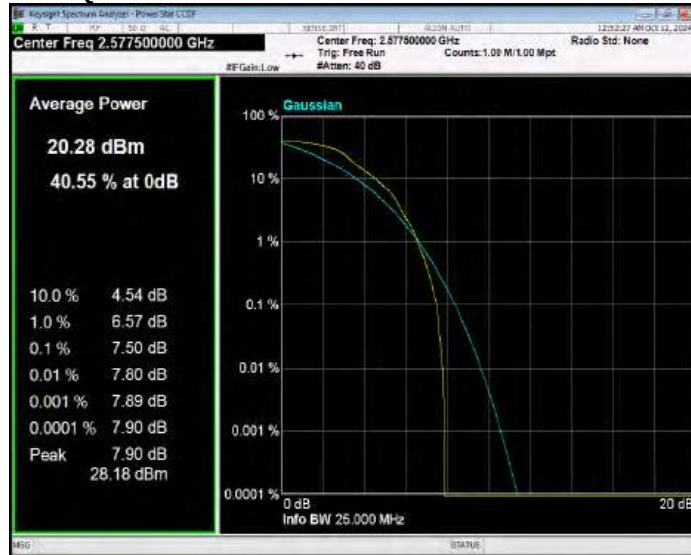
Band38 QPSK BW=15MHz Channel=38000 RB Size=1 Position=#0
