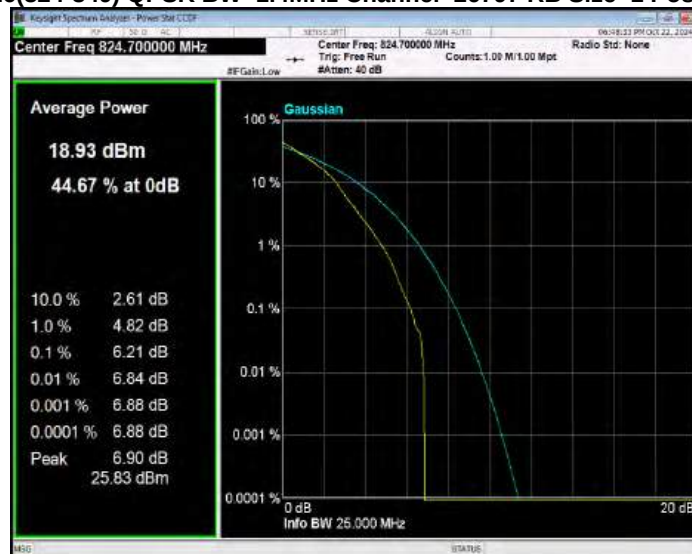
Band26(824-849) QPSK BW=1.4MHz Channel=26915 RB Size=1 Position=#0
