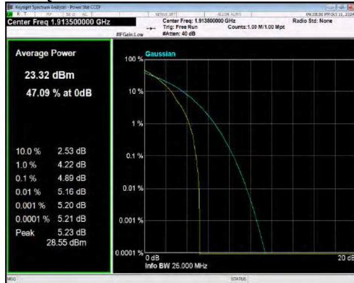
Band25 QPSK BW=5MHz Channel=26065 RB Size=1 Position=#0
