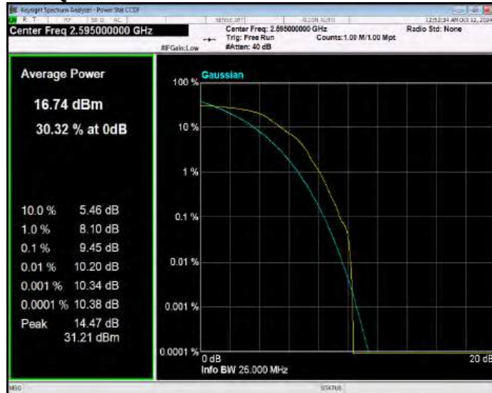
Band38 QPSK BW=15MHz Channel=38175 RB Size=1 Position=#0
