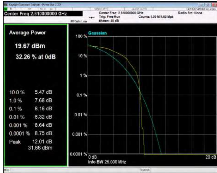
Band38 16QAM BW=5MHz Channel=37775 RB Size=1 Position=#0
