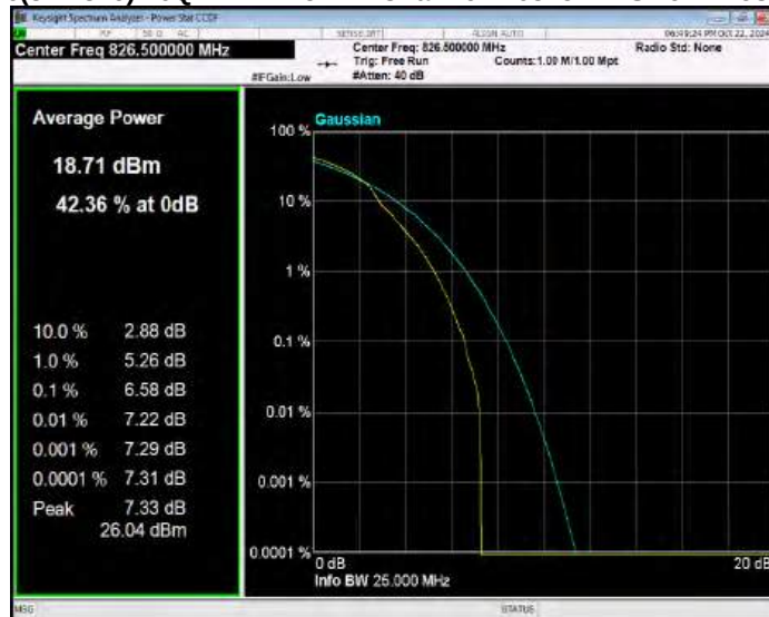
Band26(824-849) 16QAM BW=5MHz Channel=26915 RB Size=1 Position=#0
