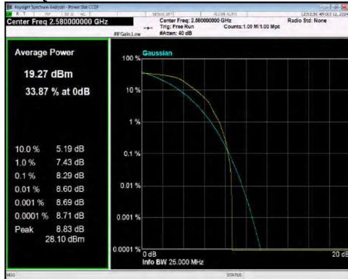
Band38 QPSK BW=20MHz Channel=38000 RB Size=1 Position=#0
