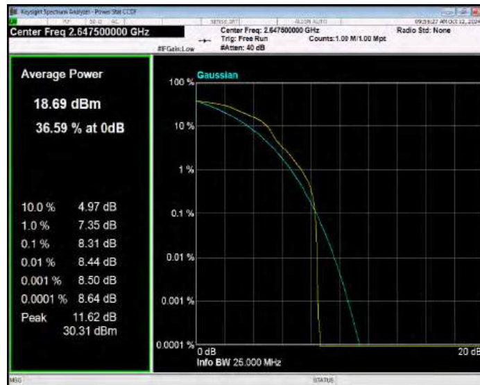
Band41(2535-2655) 16QAM BW=20MHz Channel=40140 RB Size=1 Position=#0
