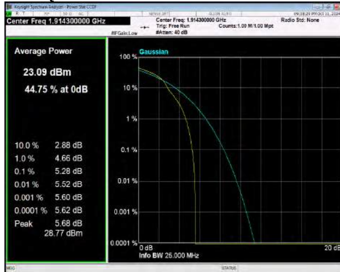
Band25 16QAM BW=10MHz Channel=26090 RB Size=1 Position=#0
