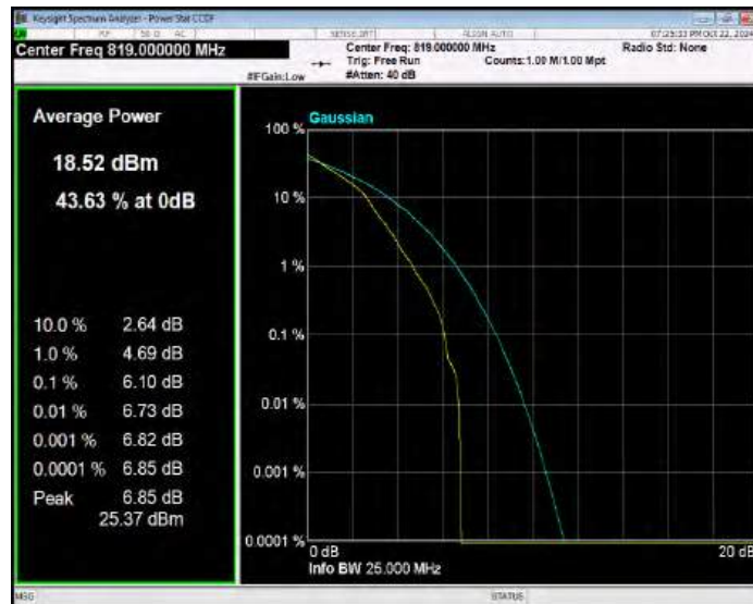
Band26(814-824) QPSK BW=3MHz Channel=26705 RB Size=1 Position=#0
