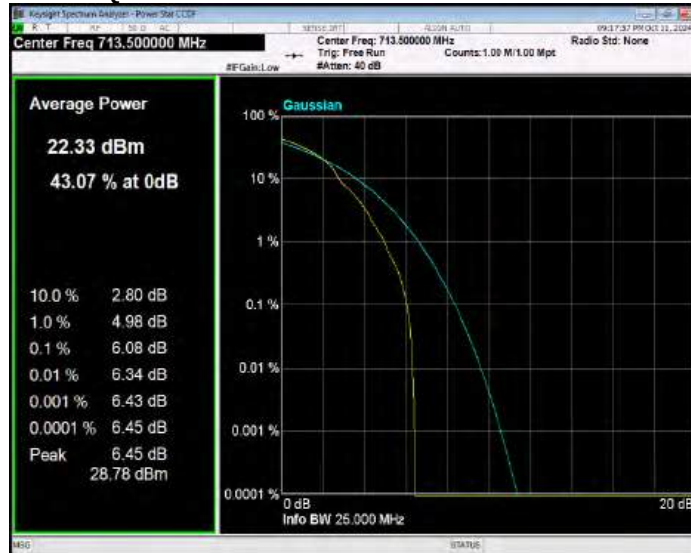
Band17 QPSK BW=10MHz Channel=23780 RB Size=1 Position=#0
