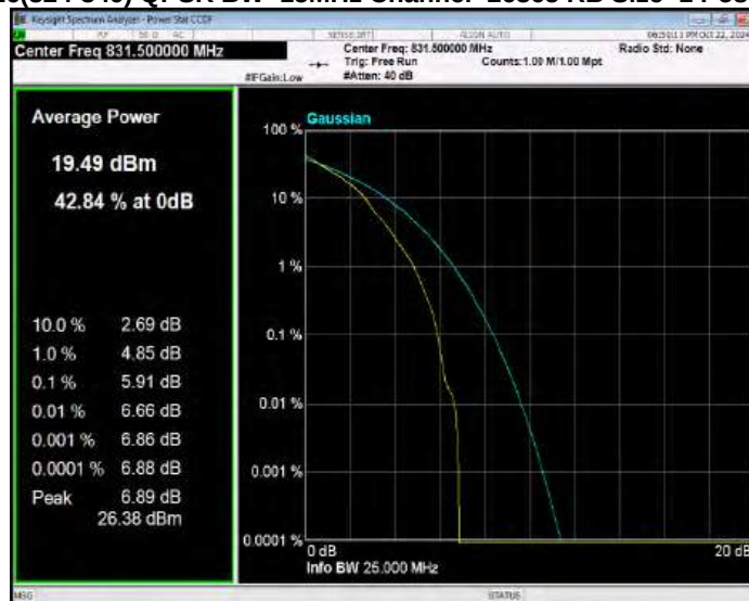
Band26(824-849) QPSK BW=15MHz Channel=26915 RB Size=1 Position=#0
