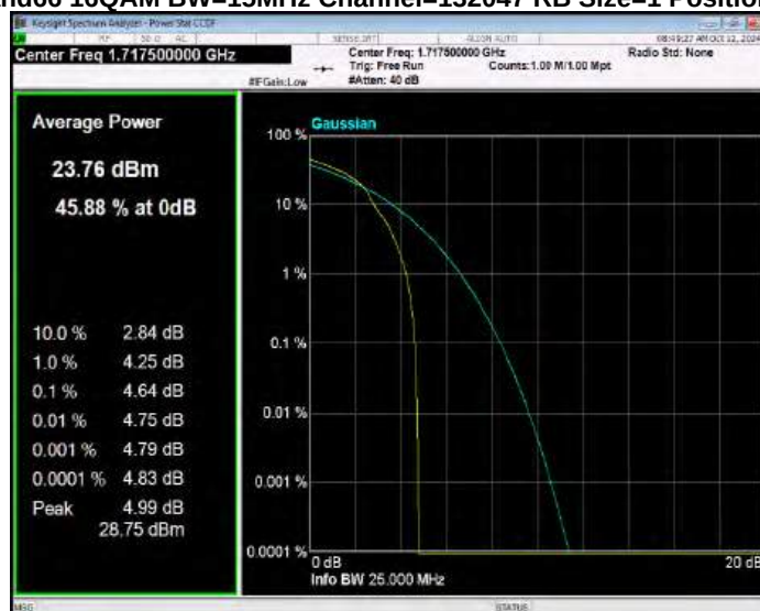
Band66 16QAM BW=15MHz Channel=132322 RB Size=1 Position=#0
