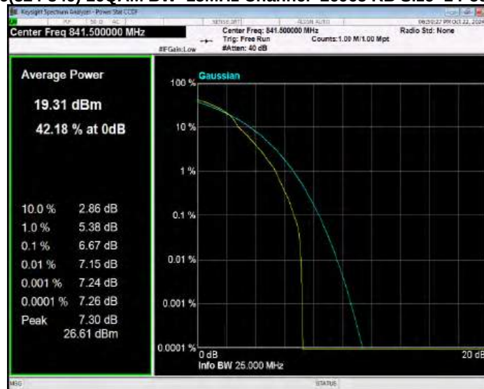
Band26(824-849) 16QAM BW=3MHz Channel=26805 RB Size=1 Position=#0
