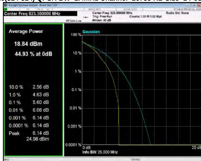
Band26(814-824) QPSK BW=10MHz Channel=26740 RB Size=1 Position=#0
