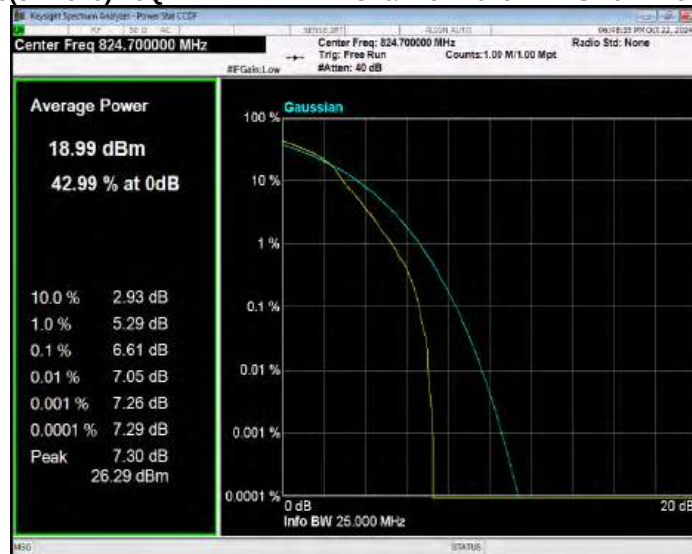
Band26(824-849) 16QAM BW=1.4MHz Channel=26915 RB Size=1 Position=#0
