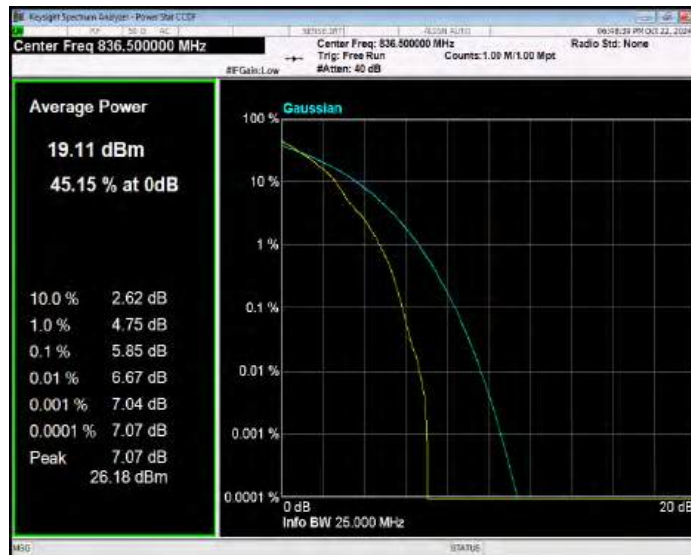
Band26(824-849) QPSK BW=1.4MHz Channel=27033 RB Size=1 Position=#0
