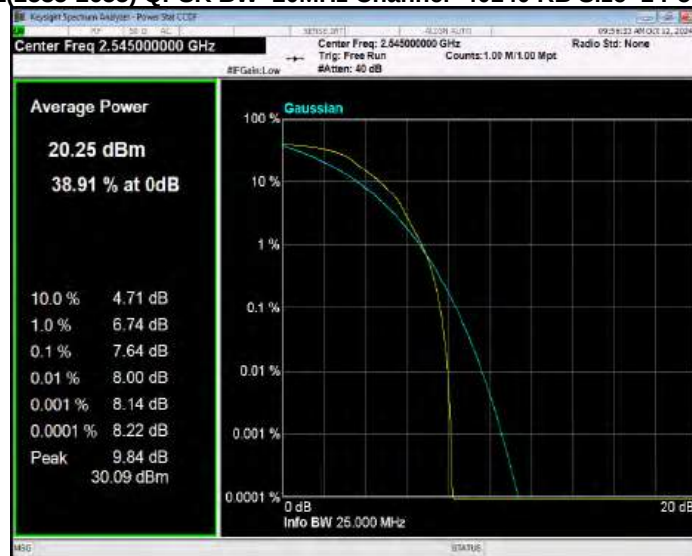
Band41(2535-2655) QPSK BW=20MHz Channel=40640 RB Size=1 Position=#0
