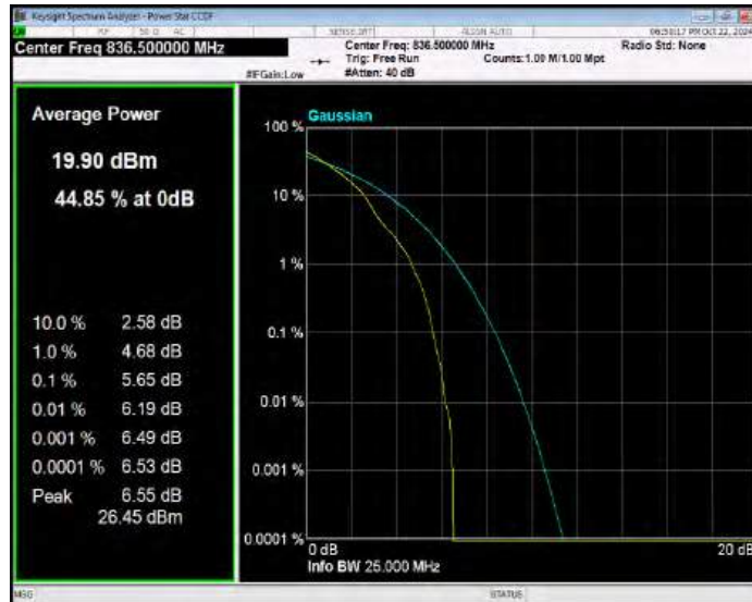
Band26(824-849) QPSK BW=15MHz Channel=26965 RB Size=1 Position=#0
