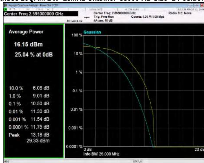
Band38 16QAM BW=15MHz Channel=38175 RB Size=1 Position=#0
