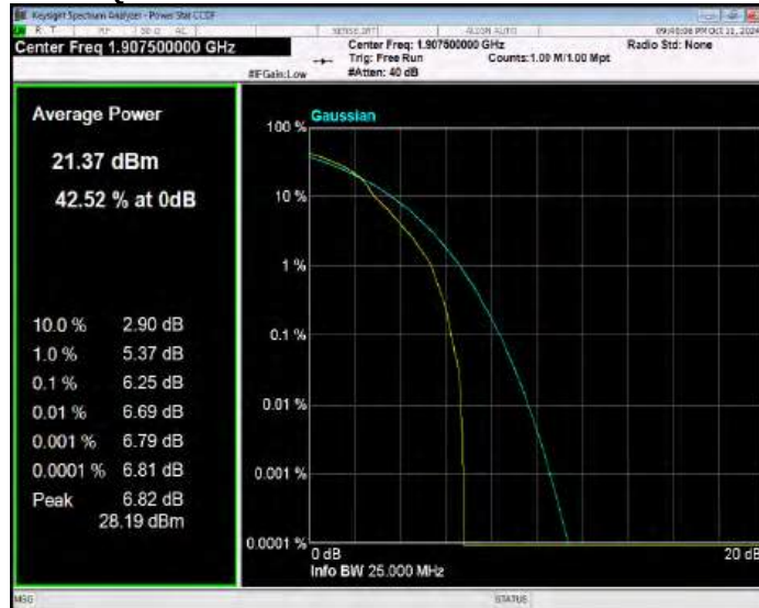
Band25 16QAM BW=20MHz Channel=26140 RB Size=1 Position=#0
