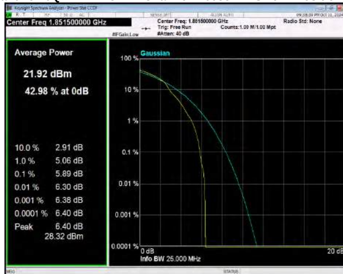
Band25 16QAM BW=3MHz Channel=26365 RB Size=1 Position=#0
