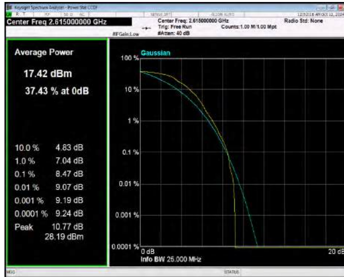
Band38 QPSK BW=15MHz Channel=37825 RB Size=1 Position=#0
