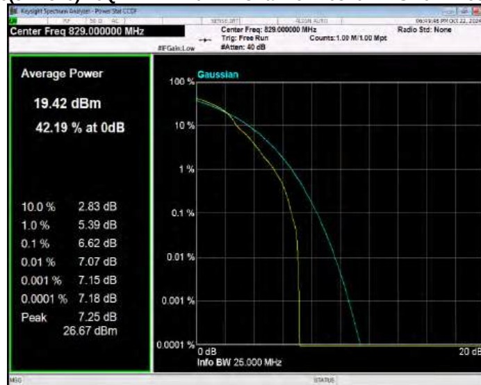
Band26(824-849) 16QAM BW=10MHz Channel=26915 RB Size=1 Position=#0
