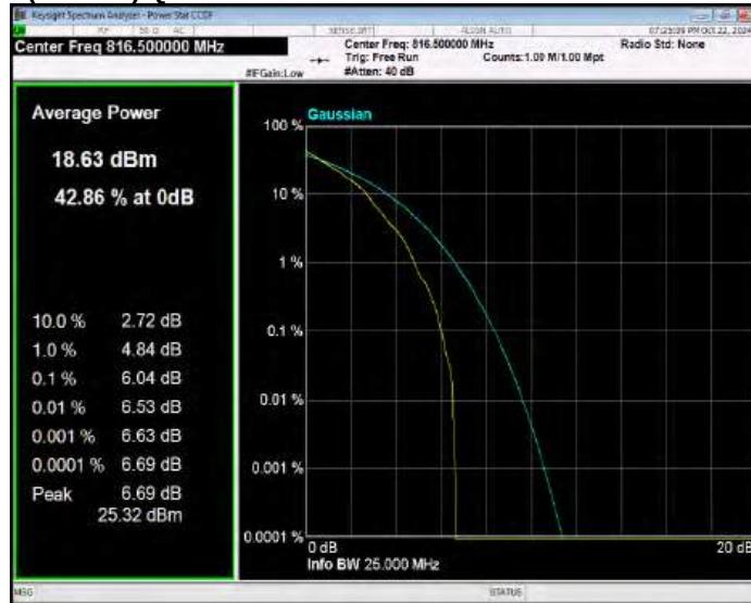
Band26(814-824) QPSK BW=5MHz Channel=26740 RB Size=1 Position=#0
