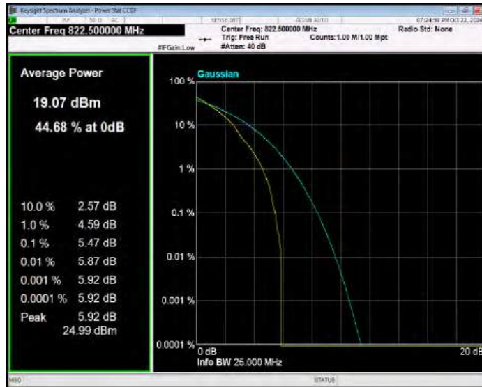
Band26(814-824) QPSK BW=5MHz Channel=26715 RB Size=1 Position=#0
