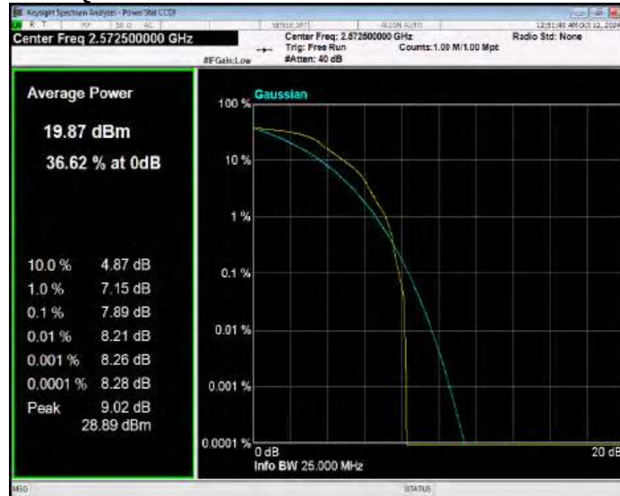
Band38 QPSK BW=5MHz Channel=38000 RB Size=1 Position=#0
