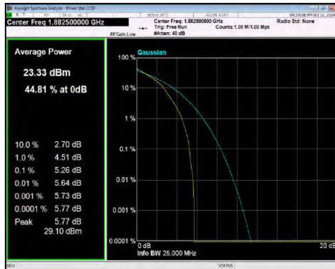
Band25 QPSK BW=5MHz Channel=26665 RB Size=1 Position=#0
