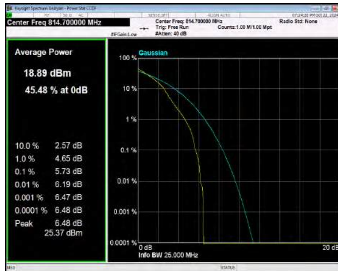
Band26(814-824) QPSK BW=1.4MHz Channel=26740 RB Size=1 Position=#0
