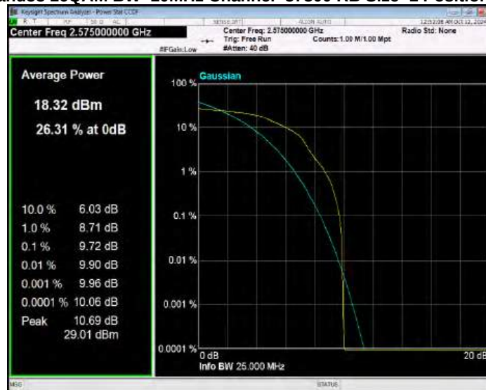
Band38 16QAM BW=10MHz Channel=38000 RB Size=1 Position=#0
