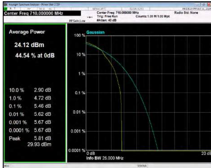
Band17 16QAM BW=10MHz Channel=23800 RB Size=1 Position=#0
