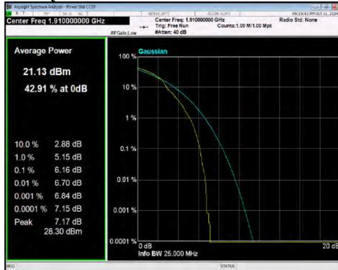
Band25 16QAM BW=15MHz Channel=26115 RB Size=1 Position=#0
