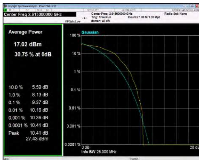
Band38 16QAM BW=15MHz Channel=37825 RB Size=1 Position=#0
