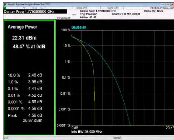
Band66 QPSK BW=10MHz Channel=132022 RB Size=1 Position=#0
