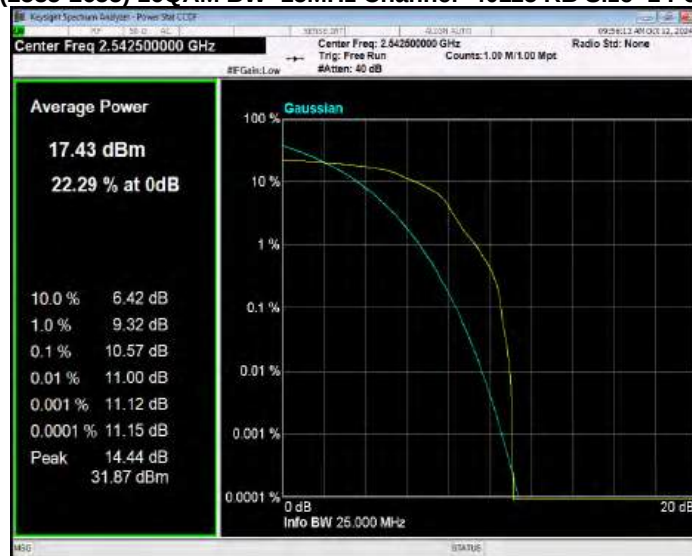
Band41(2535-2655) 16QAM BW=15MHz Channel=40640 RB Size=1 Position=#0
