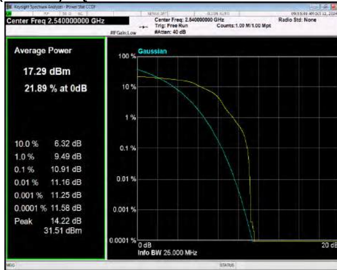
Band41(2535-2655) 16QAM BW=10MHz Channel=40640 RB Size=1 Position=#0
