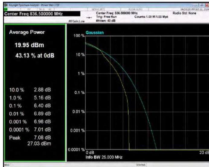
Band26(824-849) 16QAM BW=15MHz Channel=26965 RB Size=1 Position=#0
