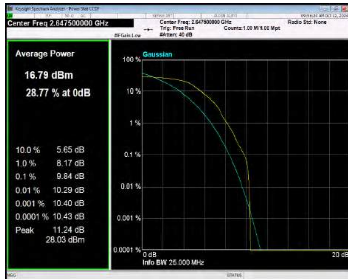
Band41(2535-2655) QPSK BW=20MHz Channel=40140 RB Size=1 Position=#0
