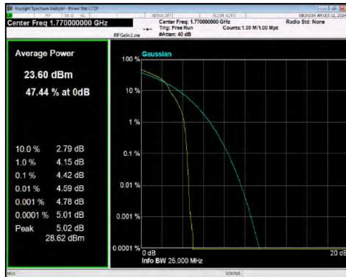
Band66 16QAM BW=3MHz Channel=131987 RB Size=1 Position=#0
