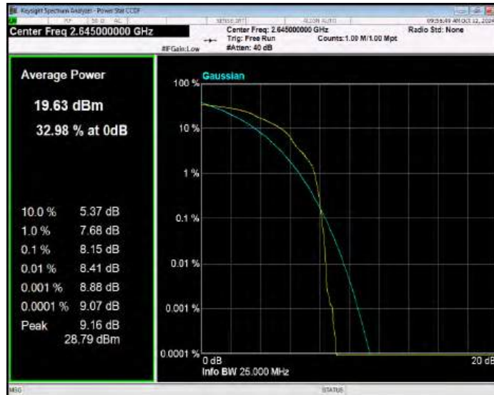
Band41(2535-2655) 16QAM BW=5MHz Channel=40065 RB Size=1 Position=#0
