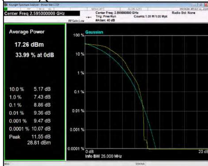
Band41(2535-2655) QPSK BW=20MHz Channel=41140 RB Size=1 Position=#0
