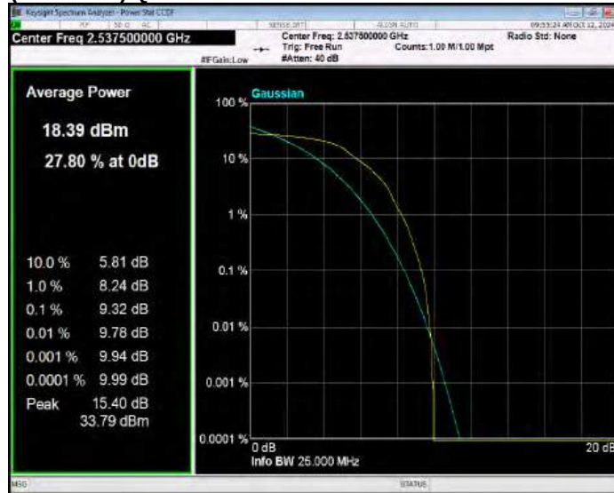
Band41(2535-2655) QPSK BW=5MHz Channel=40640 RB Size=1 Position=#0
