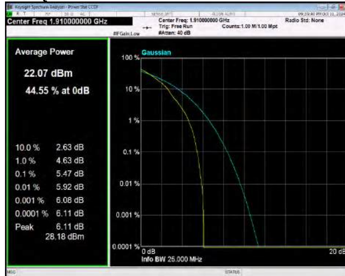
Band25 QPSK BW=15MHz Channel=26115 RB Size=1 Position=#0
