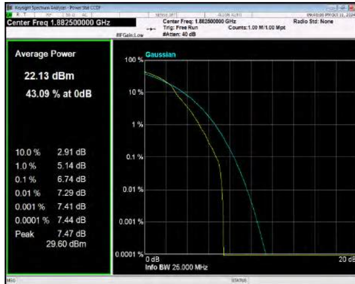
Band25 16QAM BW=15MHz Channel=26615 RB Size=1 Position=#0
