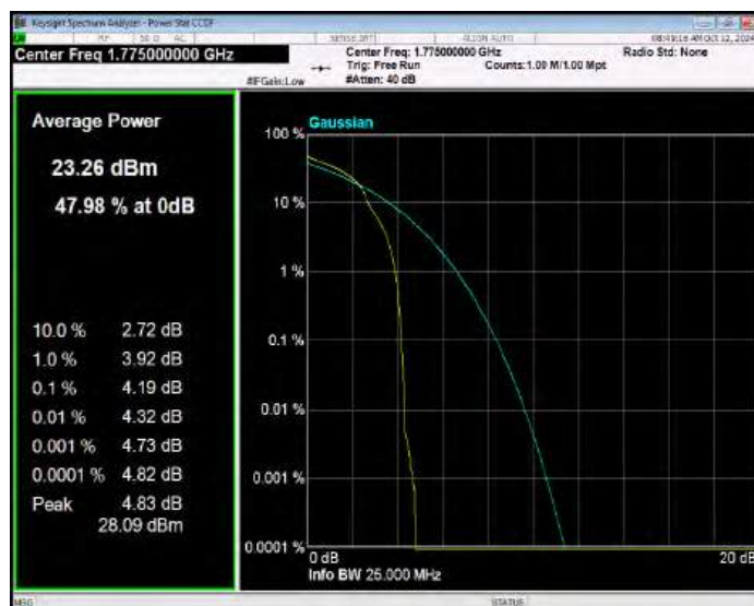
Band66 16QAM BW=15MHz Channel=132047 RB Size=1 Position=#0
