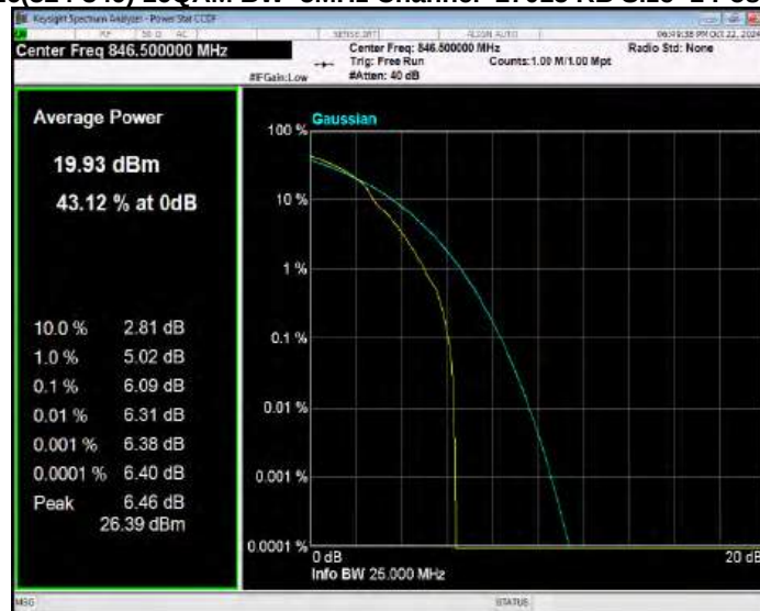
Band26(824-849) QPSK BW=1.4MHz Channel=26797 RB Size=1 Position=#0
