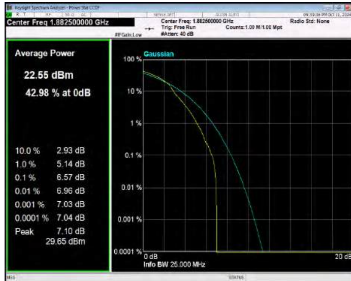
Band25 16QAM BW=10MHz Channel=26640 RB Size=1 Position=#0
