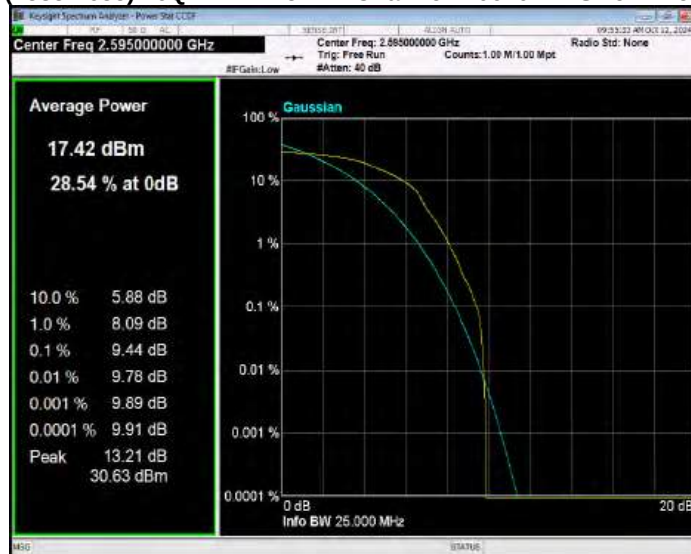
Band41(2535-2655) 16QAM BW=5MHz Channel=41215 RB Size=1 Position=#0
