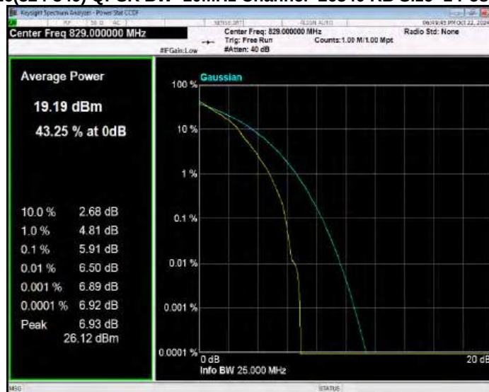
Band26(824-849) QPSK BW=10MHz Channel=26915 RB Size=1 Position=#0
