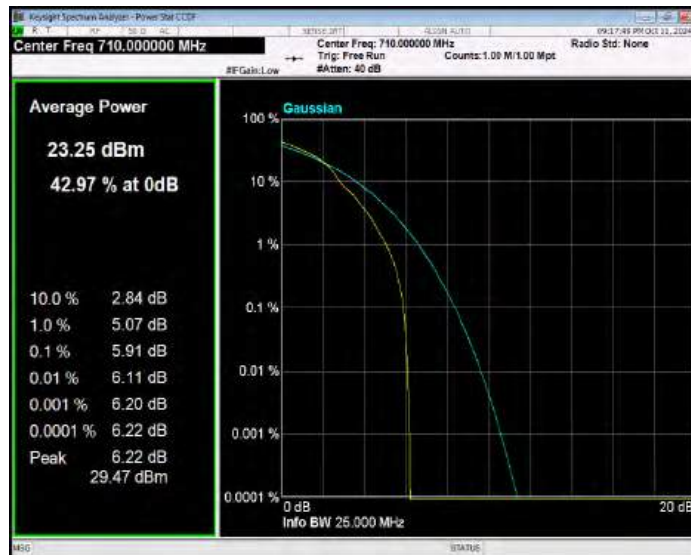
Band17 16QAM BW=5MHz Channel=23825 RB Size=1 Position=#0
