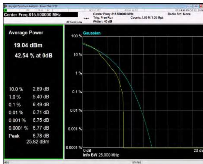
Band26(814-824) 16QAM BW=3MHz Channel=26740 RB Size=1 Position=#0
