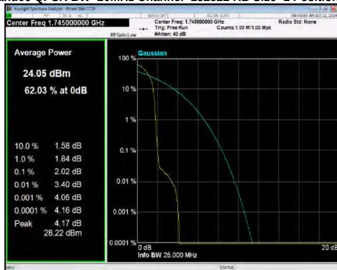
Band66 QPSK BW=20MHz Channel=132572 RB Size=1 Position=#0
