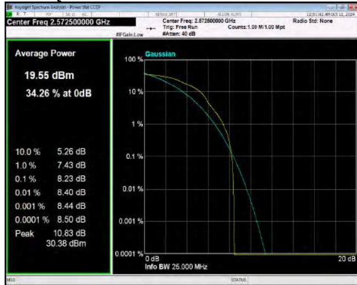
Band38 16QAM BW=5MHz Channel=38000 RB Size=1 Position=#0
