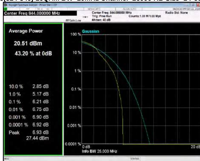
Band26(824-849) 16QAM BW=15MHz Channel=26865 RB Size=1 Position=#0
