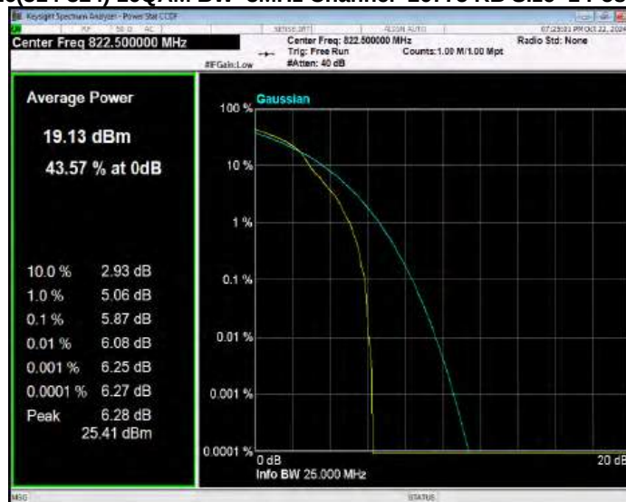
Band26(814-824) 16QAM BW=5MHz Channel=26715 RB Size=1 Position=#0
