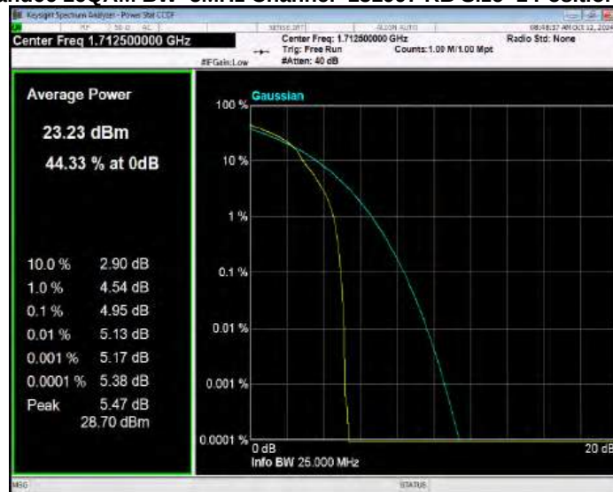
Band66 16QAM BW=5MHz Channel=132322 RB Size=1 Position=#0
