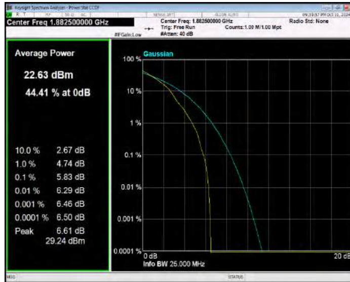
Band25 QPSK BW=15MHz Channel=26615 RB Size=1 Position=#0
