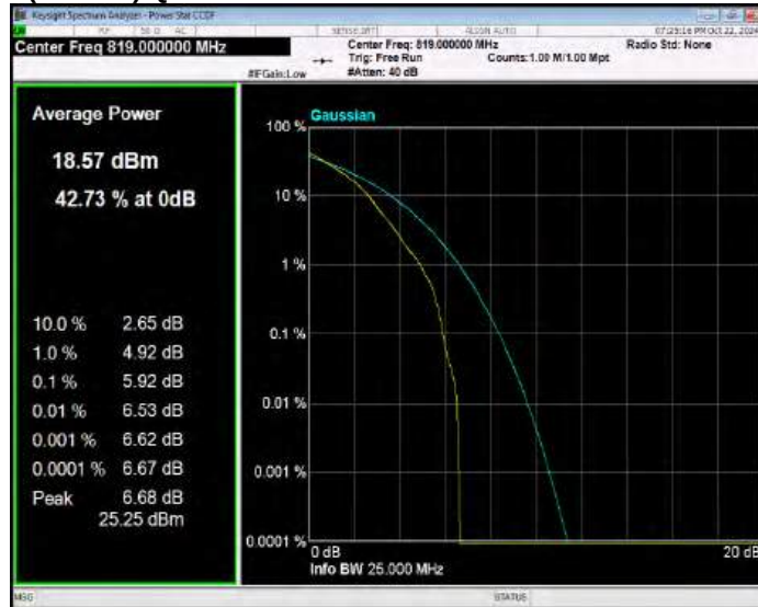
Band26(814-824) QPSK BW=5MHz Channel=26765 RB Size=1 Position=#0
