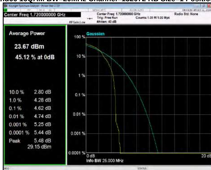
Band66 16QAM BW=20MHz Channel=132322 RB Size=1 Position=#0
