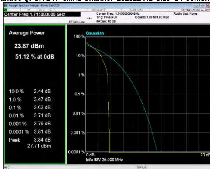
Band66 QPSK BW=3MHz Channel=132657 RB Size=1 Position=#0
