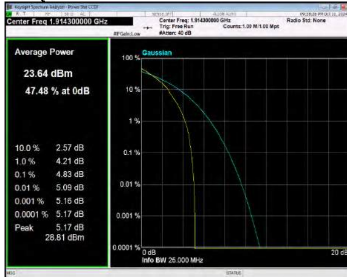
Band25 QPSK BW=10MHz Channel=26090 RB Size=1 Position=#0
