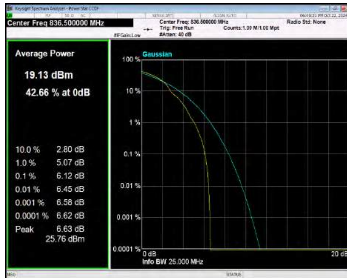
Band26(824-849) 16QAM BW=5MHz Channel=27015 RB Size=1 Position=#0
