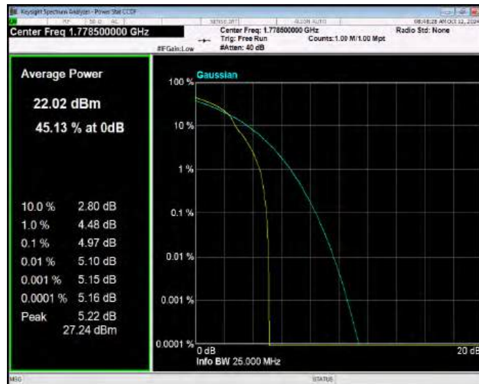
Band66 16QAM BW=5MHz Channel=131997 RB Size=1 Position=#0
