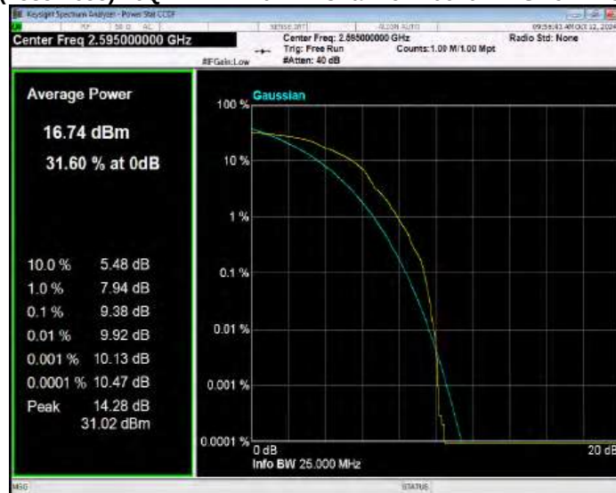
Band41(2535-2655) 16QAM BW=20MHz Channel=41140 RB Size=1 Position=#0
