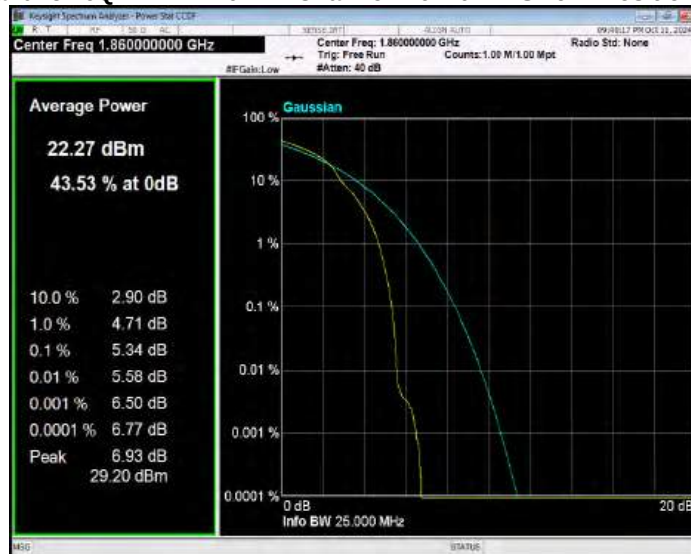
Band25 16QAM BW=20MHz Channel=26365 RB Size=1 Position=#0
