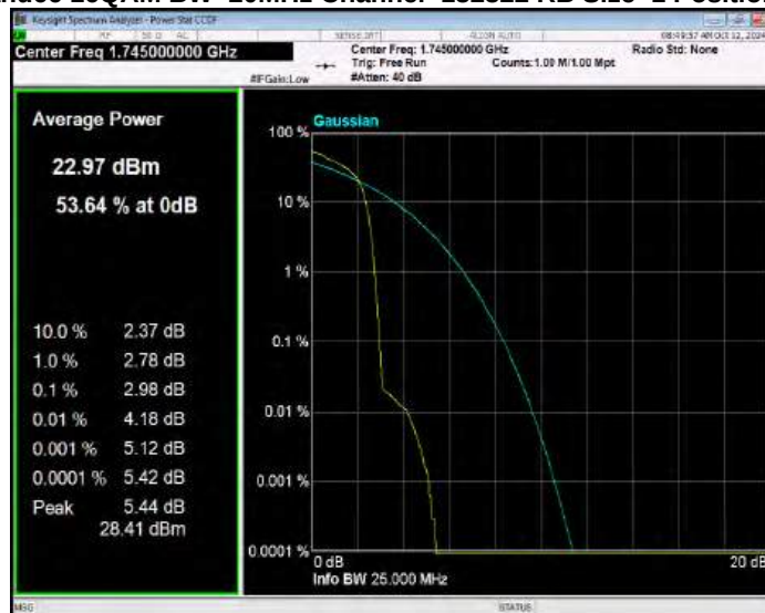
Band66 16QAM BW=20MHz Channel=132572 RB Size=1 Position=#0
