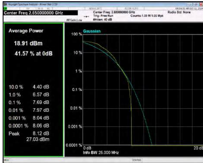
Band41(2535-2655) QPSK BW=15MHz Channel=40115 RB Size=1 Position=#0
