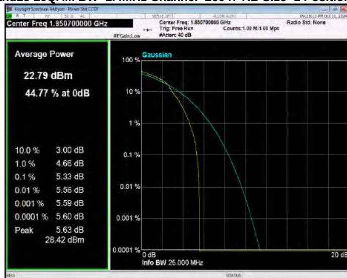
Band25 16QAM BW=1.4MHz Channel=26365 RB Size=1 Position=#0
