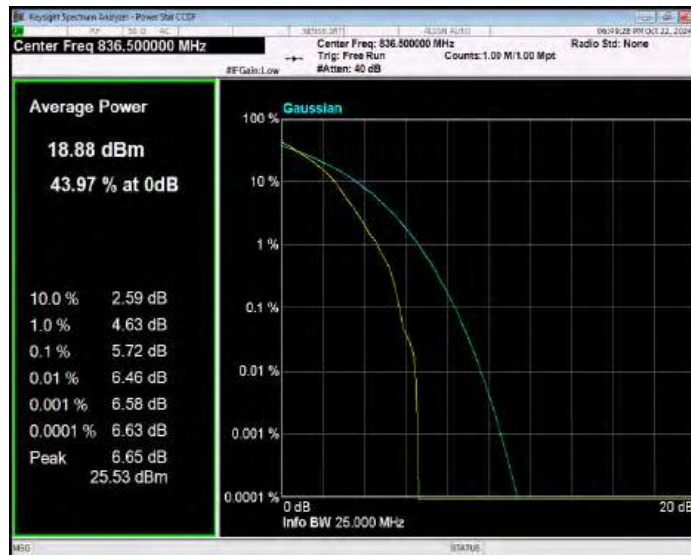
Band26(824-849) QPSK BW=5MHz Channel=27015 RB Size=1 Position=#0
