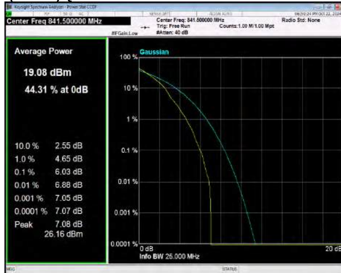
Band26(824-849) QPSK BW=3MHz Channel=26805 RB Size=1 Position=#0
