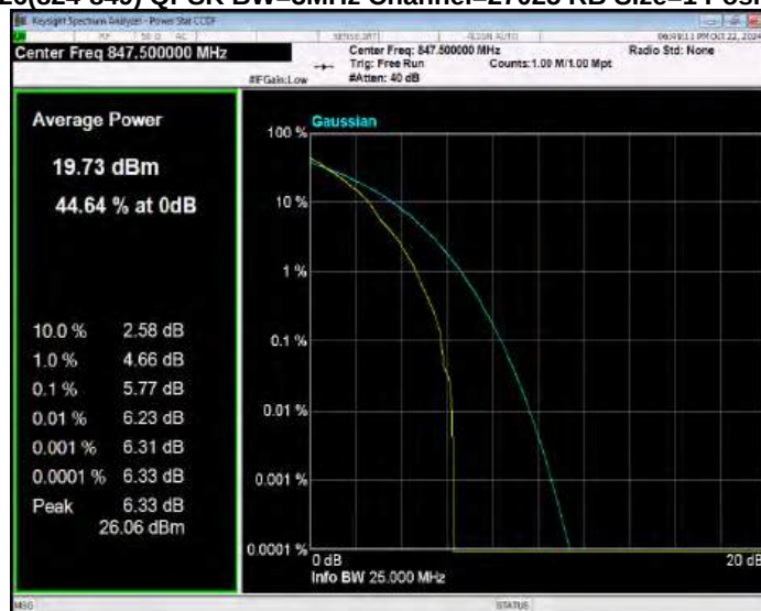
Band26(824-849) QPSK BW=5MHz Channel=26815 RB Size=1 Position=#0
