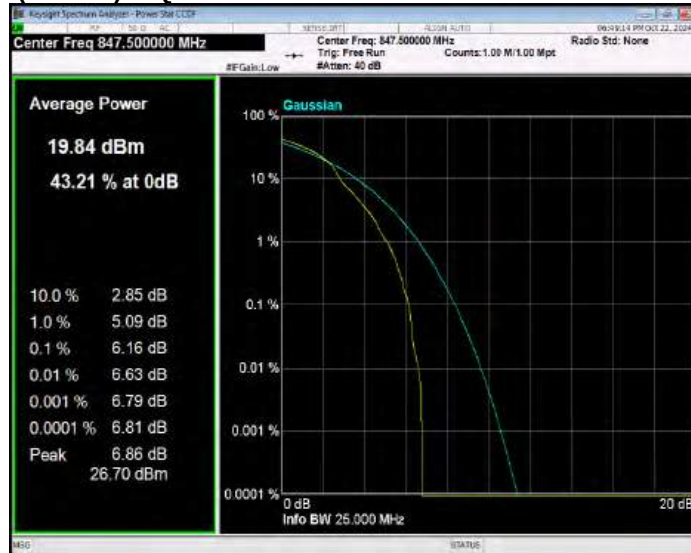
Band26(824-849) 16QAM BW=5MHz Channel=26815 RB Size=1 Position=#0
