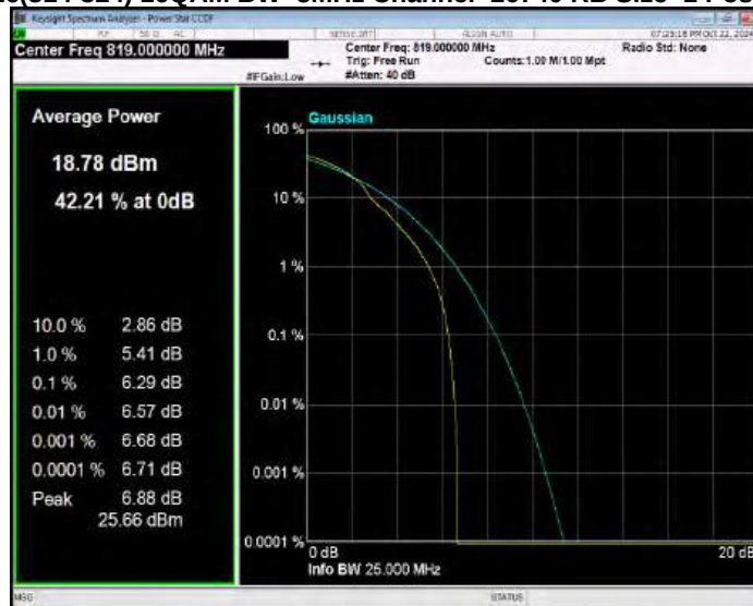
Band26(814-824) 16QAM BW=5MHz Channel=26765 RB Size=1 Position=#0
