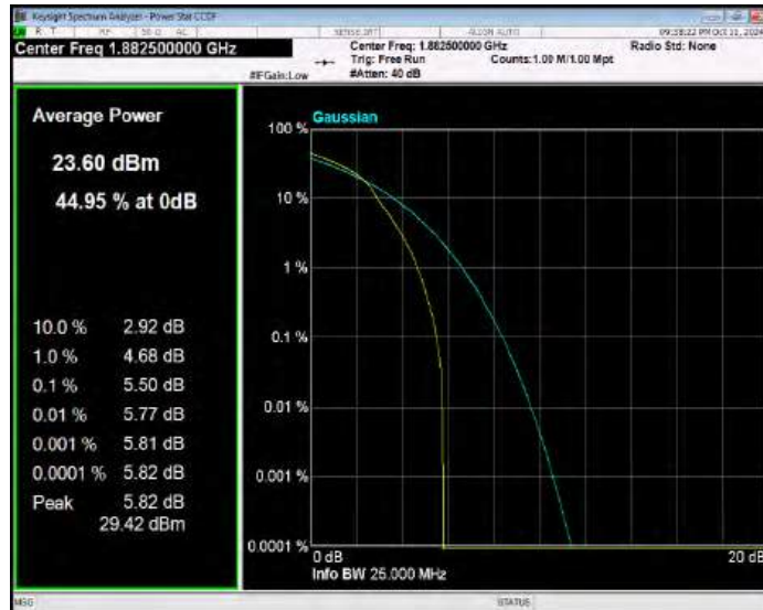
Band25 16QAM BW=1.4MHz Channel=26683 RB Size=1 Position=#0
