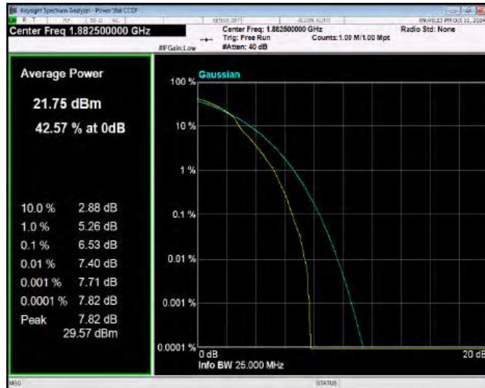
Band25 16QAM BW=20MHz Channel=26590 RB Size=1 Position=#0
