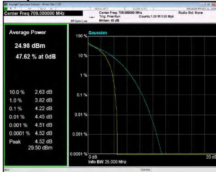
Band17 QPSK BW=10MHz Channel=23790 RB Size=1 Position=#0
