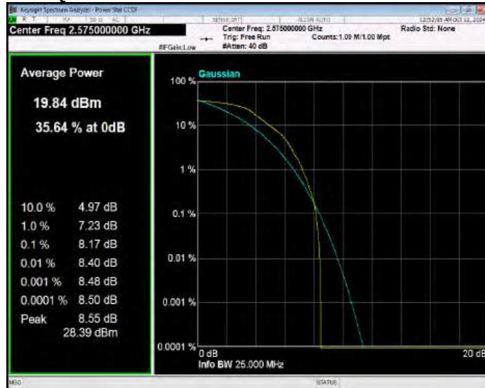
Band38 QPSK BW=10MHz Channel=38000 RB Size=1 Position=#0
