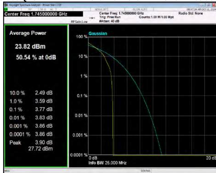
Band66 QPSK BW=1.4MHz Channel=132665 RB Size=1 Position=#0
