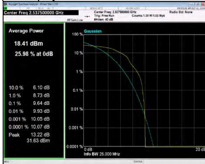
Band41(2535-2655) 16QAM BW=5MHz Channel=40640 RB Size=1 Position=#0
