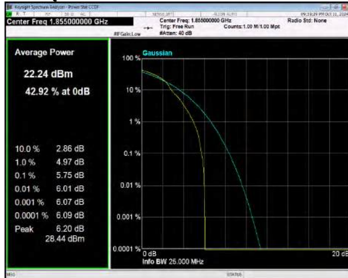
Band25 16QAM BW=10MHz Channel=26365 RB Size=1 Position=#0
