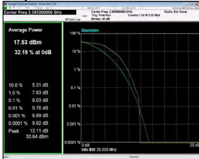
Band38 QPSK BW=10MHz Channel=38200 RB Size=1 Position=#0
