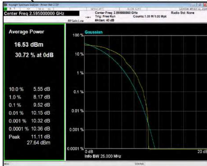
Band38 16QAM BW=20MHz Channel=38150 RB Size=1 Position=#0
