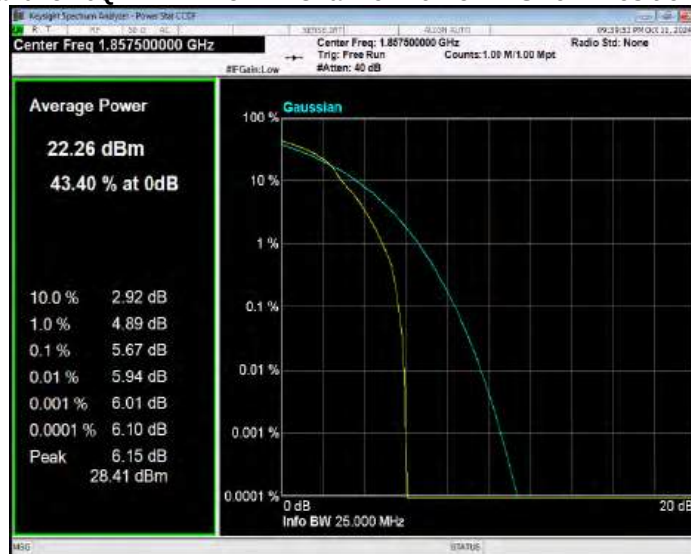
Band25 16QAM BW=15MHz Channel=26365 RB Size=1 Position=#0
