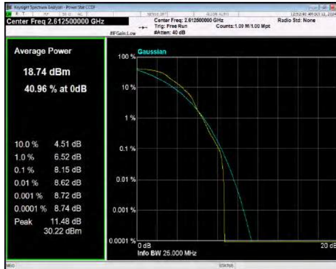
Band38 QPSK BW=20MHz Channel=37850 RB Size=1 Position=#0
