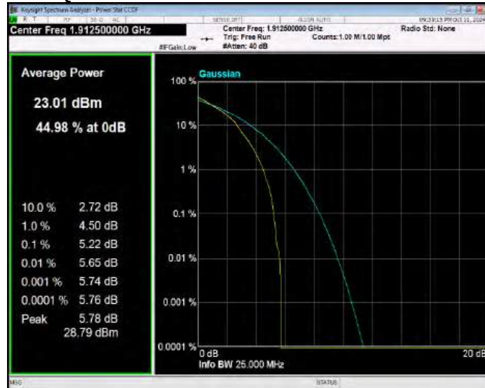
Band26(824-849) 16QAM BW=1.4MHz Channel=26797 RB Size=1 Position=#0
