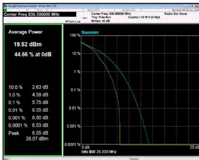
Band26(824-849) QPSK BW=10MHz Channel=26990 RB Size=1 Position=#0
