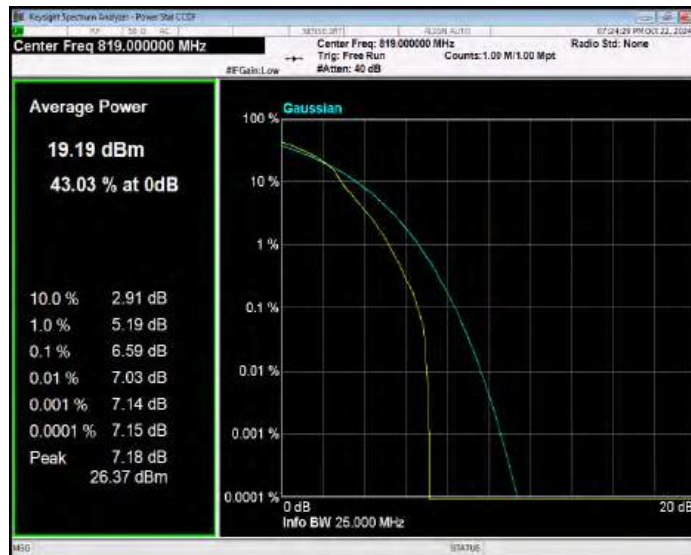
Band26(814-824) 16QAM BW=1.4MHz Channel=26783 RB Size=1 Position=#0
