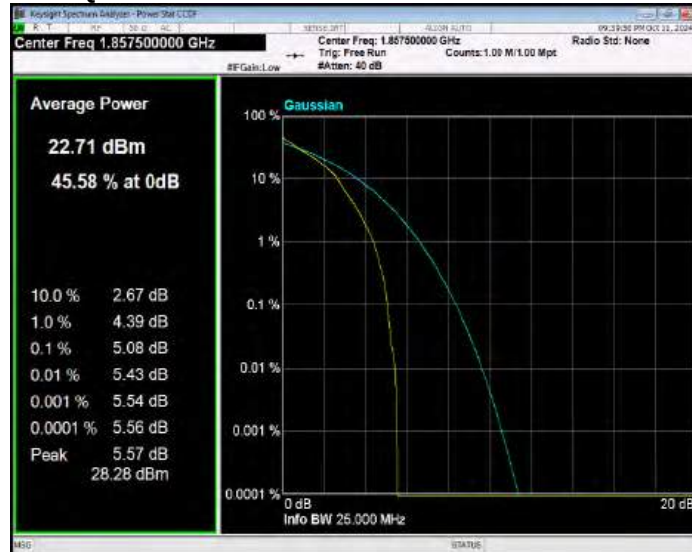
Band25 QPSK BW=15MHz Channel=26365 RB Size=1 Position=#0
