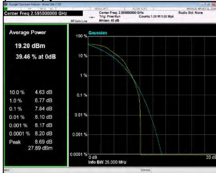
Band41(2535-2655) QPSK BW=5MHz Channel=41215 RB Size=1 Position=#0
