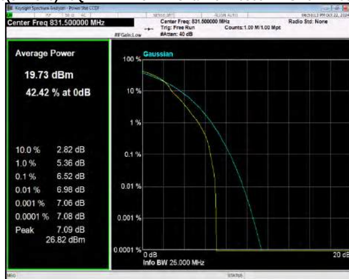
Band26(824-849) 16QAM BW=15MHz Channel=26915 RB Size=1 Position=#0
