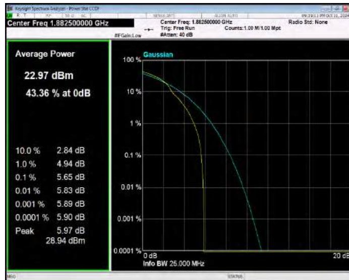
Band25 16QAM BW=5MHz Channel=26665 RB Size=1 Position=#0
