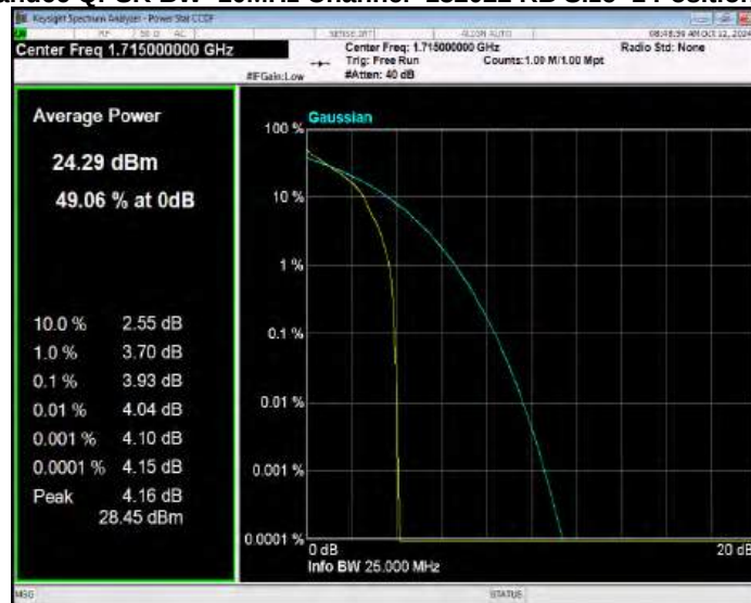
Band66 QPSK BW=10MHz Channel=132322 RB Size=1 Position=#0
