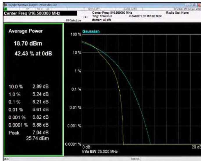
Band26(814-824) 16QAM BW=5MHz Channel=26740 RB Size=1 Position=#0
