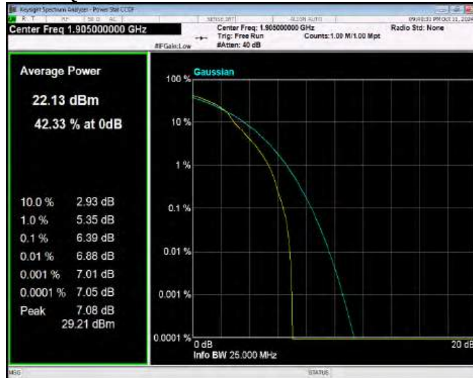
Band25 16QAM BW=3MHz Channel=26055 RB Size=1 Position=#0
