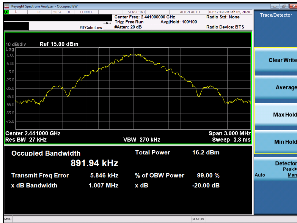
Plot 7-2. 20dB Bandwidth Plot (Bluetooth, 1Mbps – Ch. 39)
