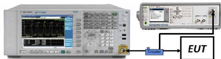
Figure 7-6. Test Instrument & Measurement Setup
