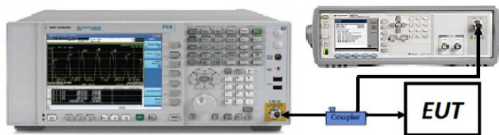
Figure 7-4. Test Instrument & Measurement Setup
