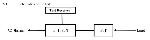
EUT: Equipment Under Test
