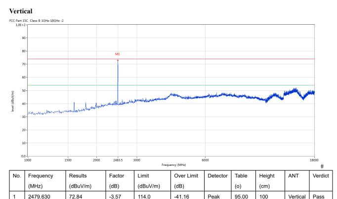
Note: (2) Emission Level = Reading Level + Antenna Factor + Cable Loss-Amplifier
