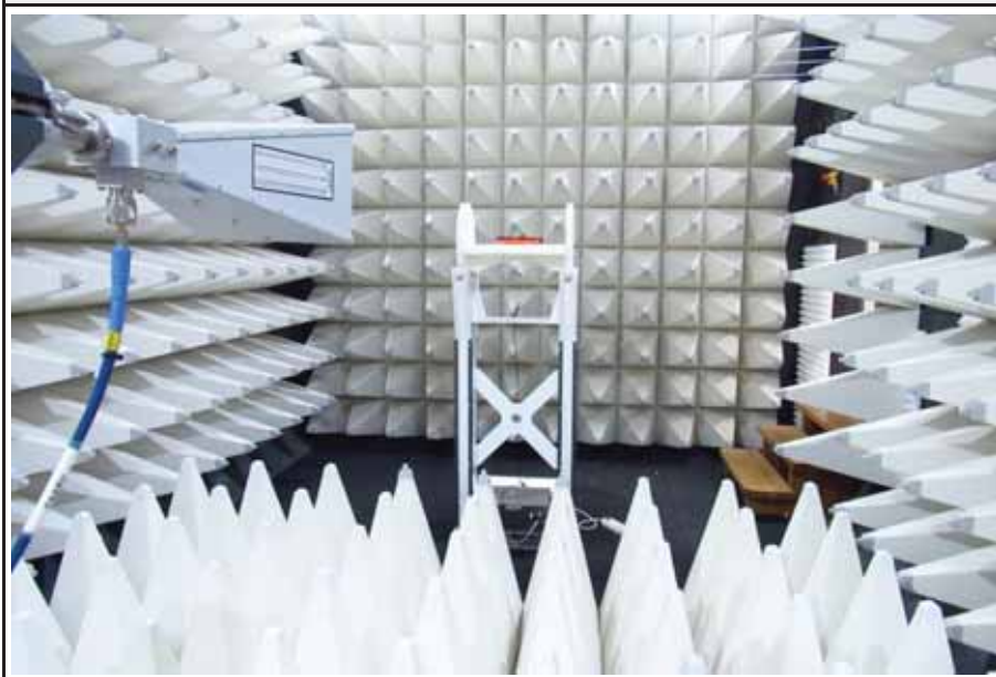
Setup for measurements above 1 GHz with Onboard antenna
