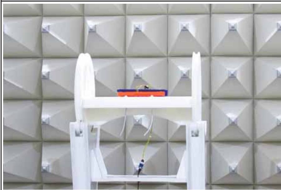
Setup for measurements above 1 GHz with Onboard antenna (2)
