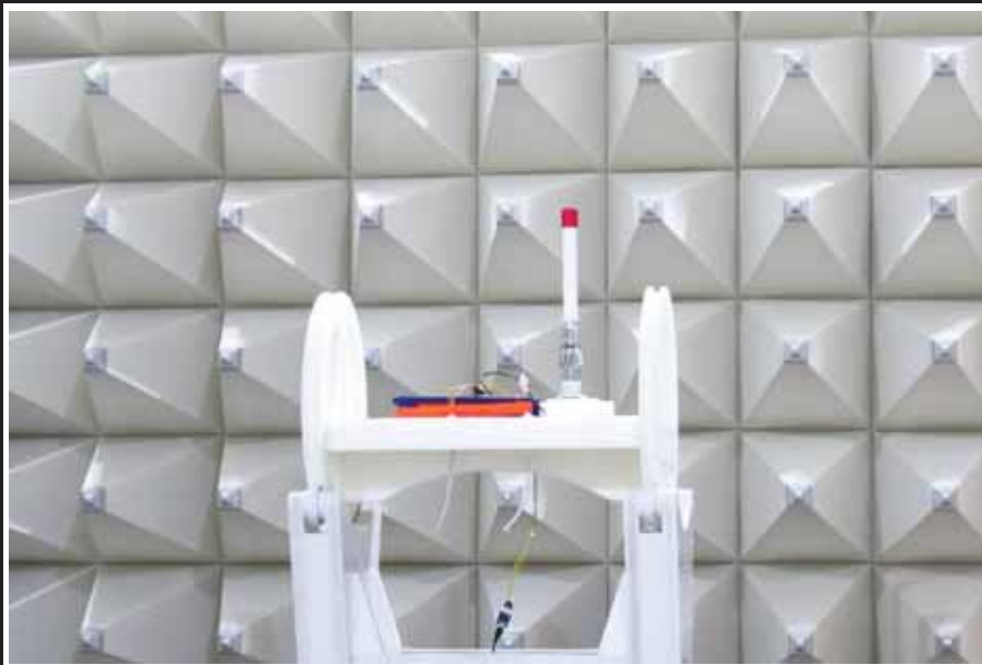
Setup for measurements above 1 GHz with antenna AA050031 (2)
