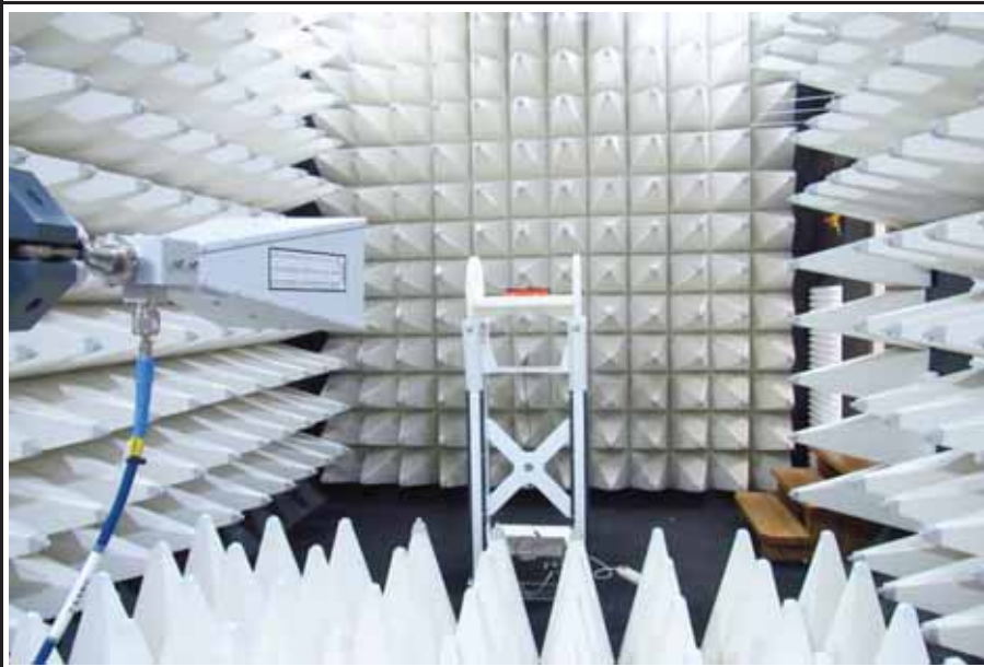
Setup for measurements above 1 GHz with antenna AA080004
