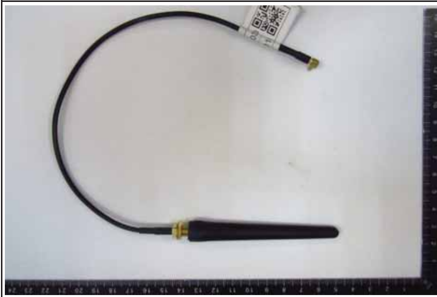
AA030018 (Sleeve antenna) with MMCX to SMA Adapter
