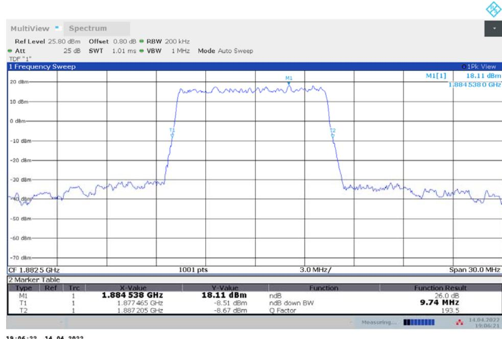
**n25,10MHz Bandwidth,DFT-s-QPSK (-26dBc BW)**
