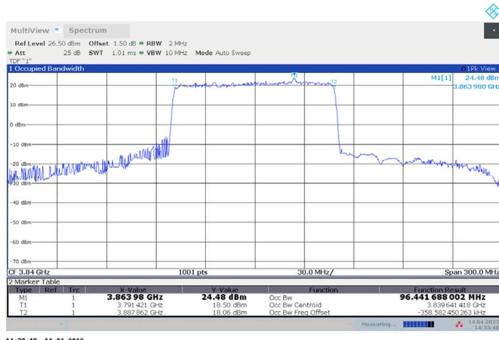
**n77H,100MHz Bandwidth,DFT-s-QPSK (99% BW)**
