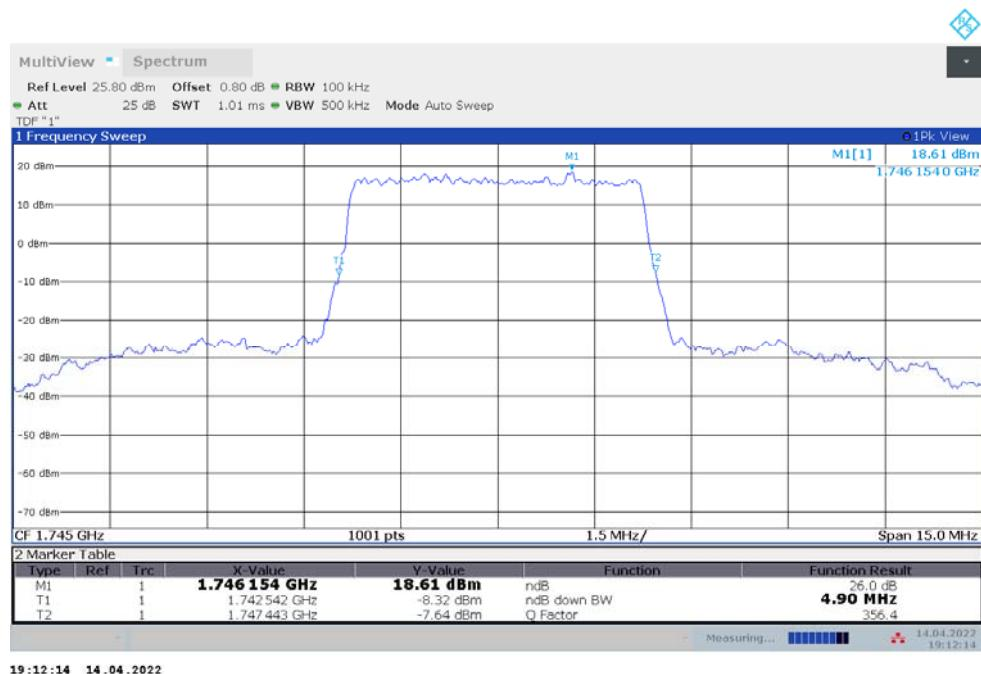
**n66,5MHz Bandwidth,DFT-s-QPSK (-26dBc BW)**
