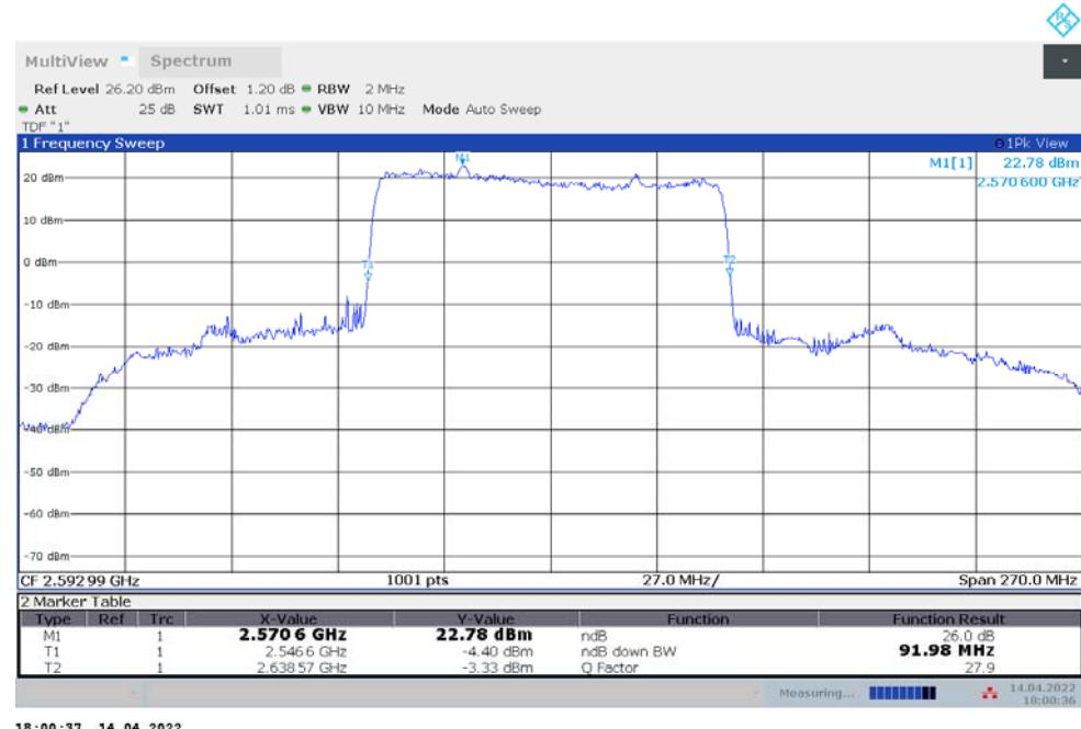
**n41,90MHz Bandwidth,DFT-s-QPSK (-26dBc BW)**
