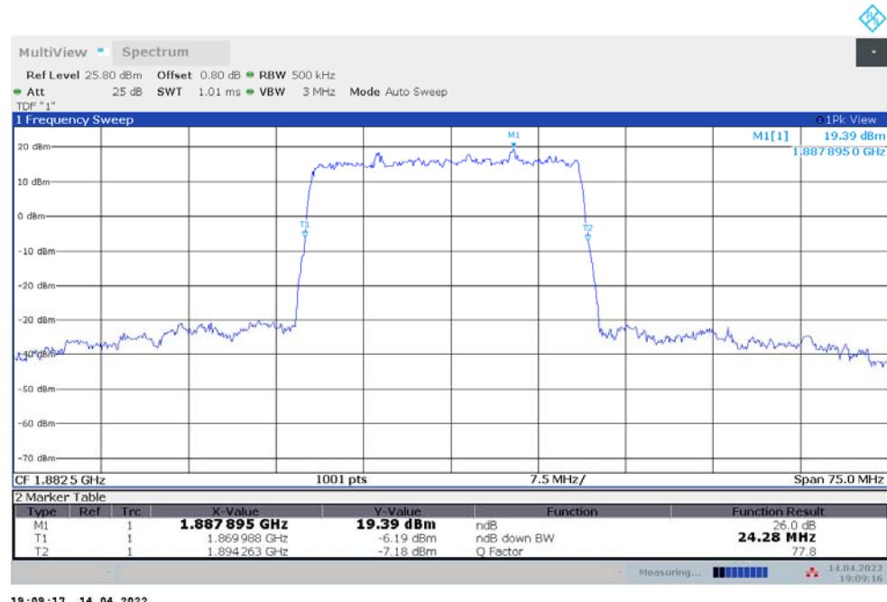
**n25,25MHz Bandwidth,DFT-s-QPSK (-26dBc BW)**
