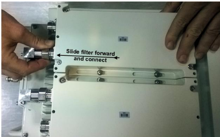
Figure 15: Align and fit second filter to connector
