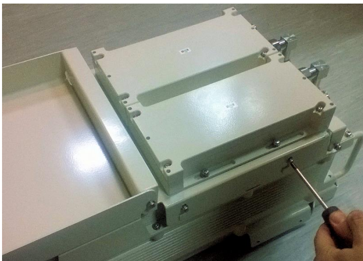
Figure 16: Tighten filter bridge screws on Sun-Shield
