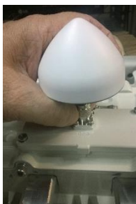
Figure 18: Attaching GPS antenna to unit
