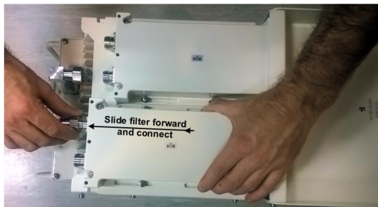
Figure 13: Align and fit filter to connector
