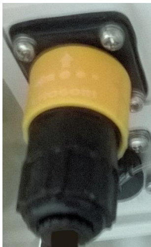
Figure 45: Power cable attached to AirHarmony-4000
