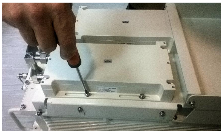
Figure 14: Tighten screws on filter
