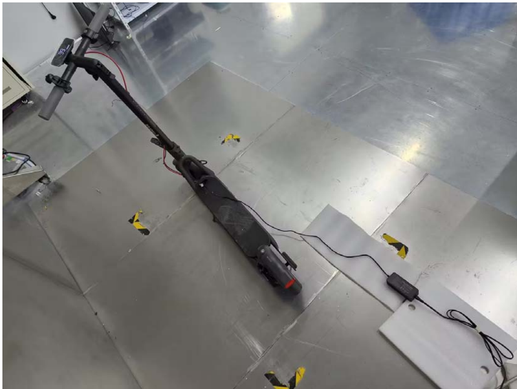
Conducted Emissions Side View- SPU:V40Pro
