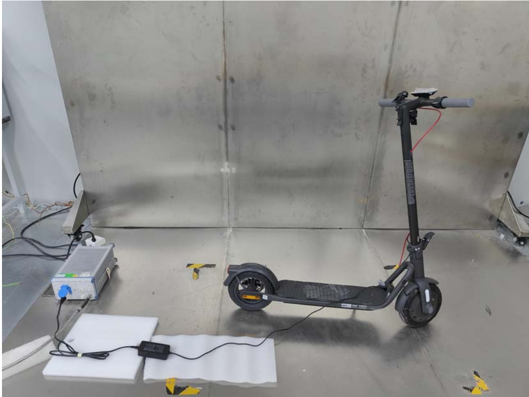
Conducted Emissions Side View- SPU:V40Pro
