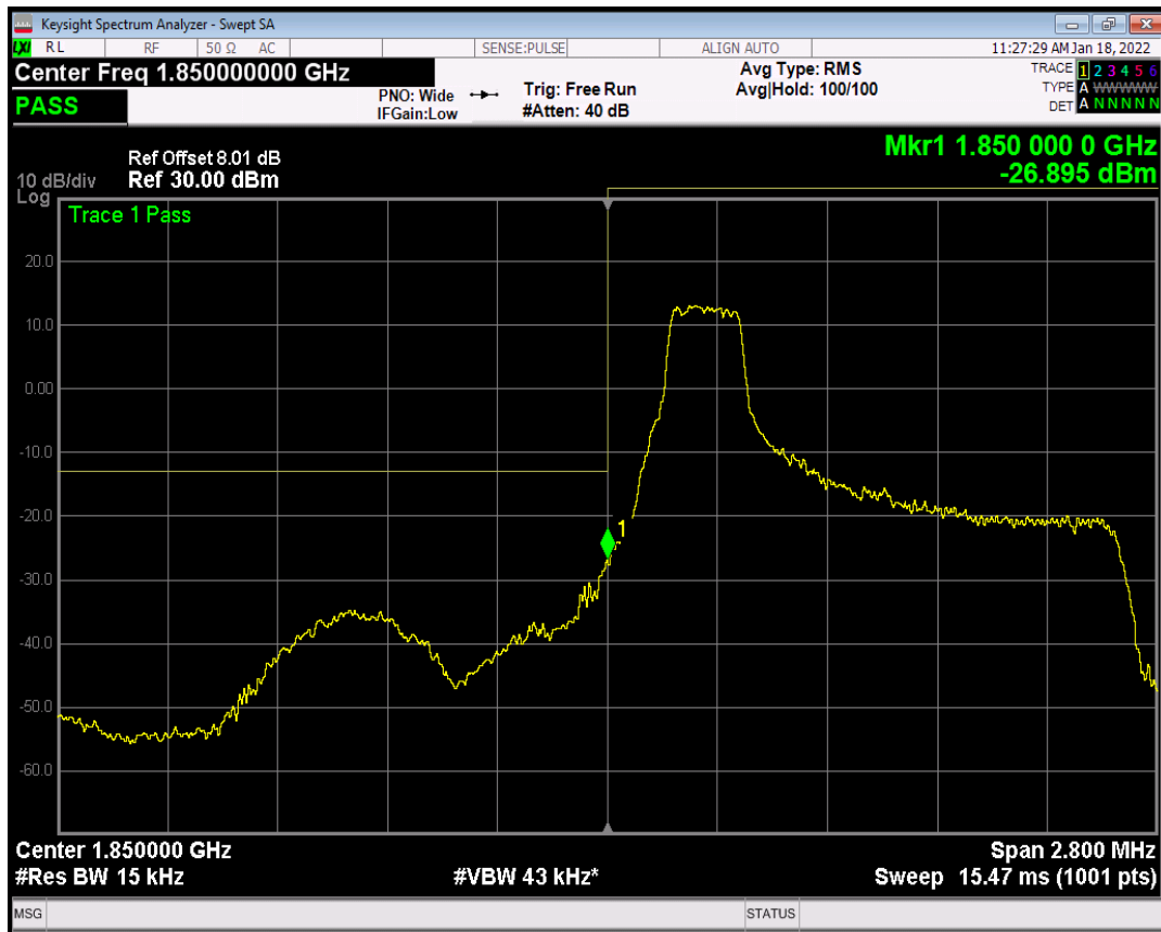
Band2 QAM16 BW=10MHz Channel=19150 RB Size=50 Position=#0
