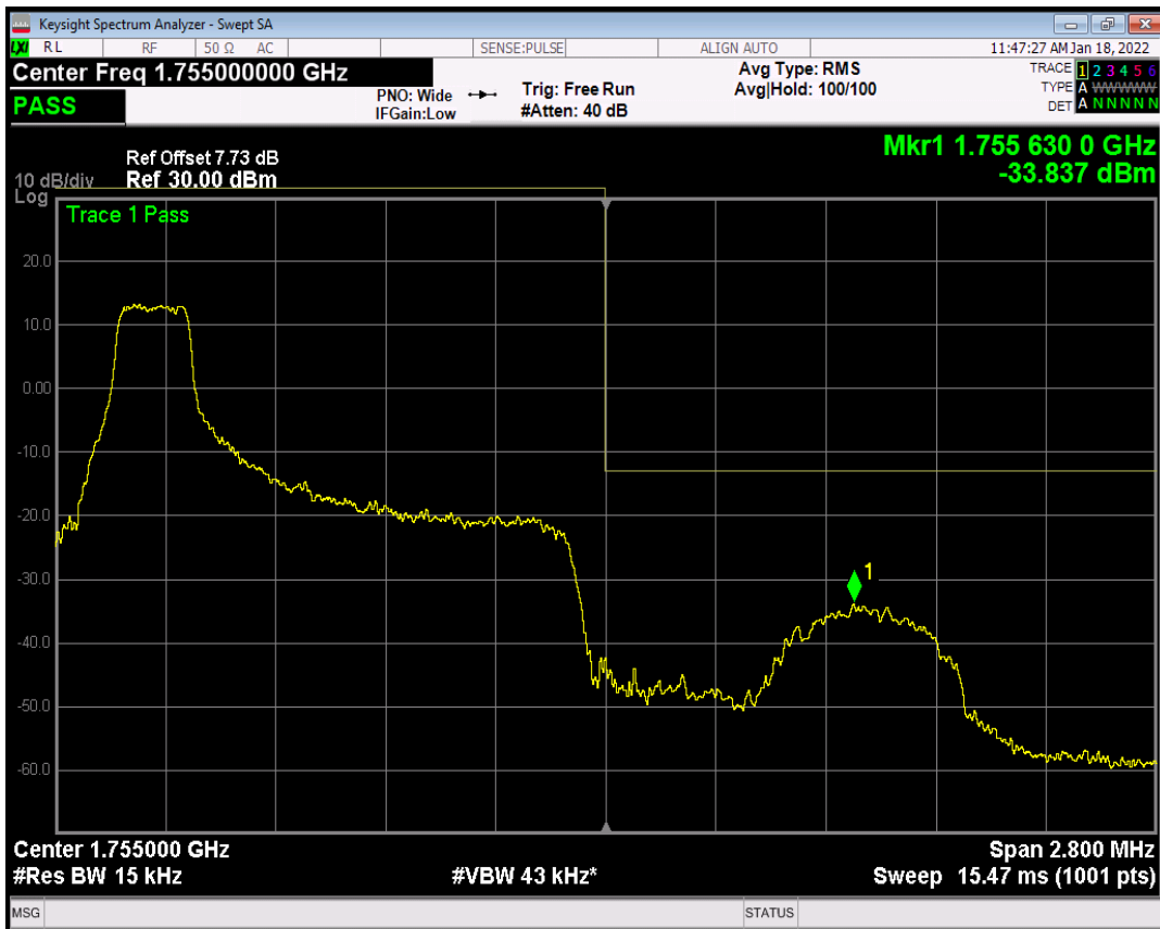
Band4 QAM16 BW=1.4MHz Channel=19957 RB Size=1 Position=#0
