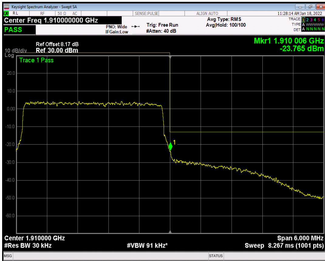
Band2 QAM16 BW=5MHz Channel=18625 RB Size=1 Position=#0
