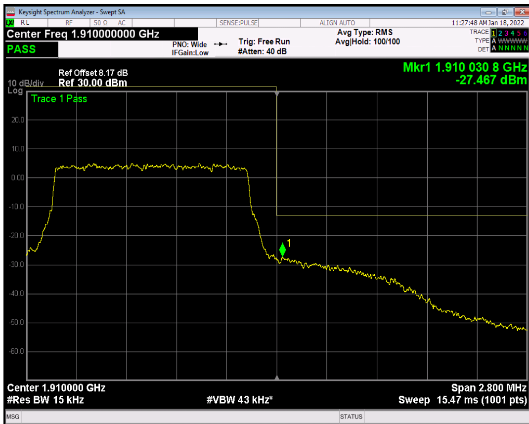
Band2 QAM16 BW=1.4MHz Channel=19193 RB Size=1 Position=#0
