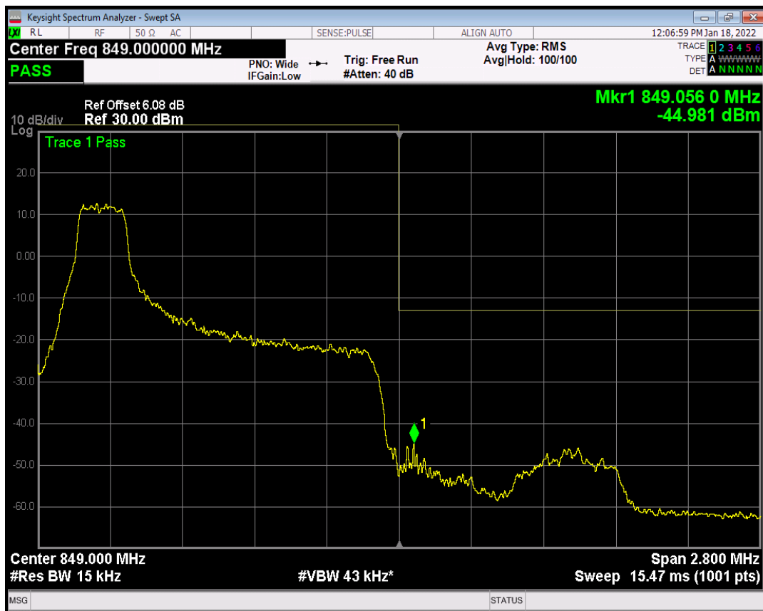
Band5 QAM16 BW=1.4MHz Channel=20407 RB Size=1 Position=#0
