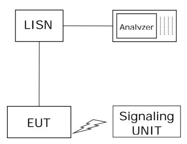
Setup in the shielded room for conducted measurements at AC mains port
