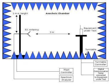
Remark: Depending on the frequency range suitable antenna types, attenuators or preamplifiers are used.
