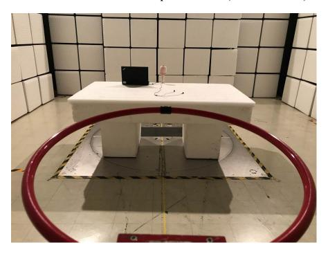
Radiated Emissions - Parallel View (9 kHz - 30 MHz)
