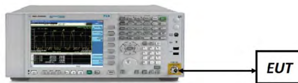
Figure 7-4. Test Instrument & Measurement Setup
