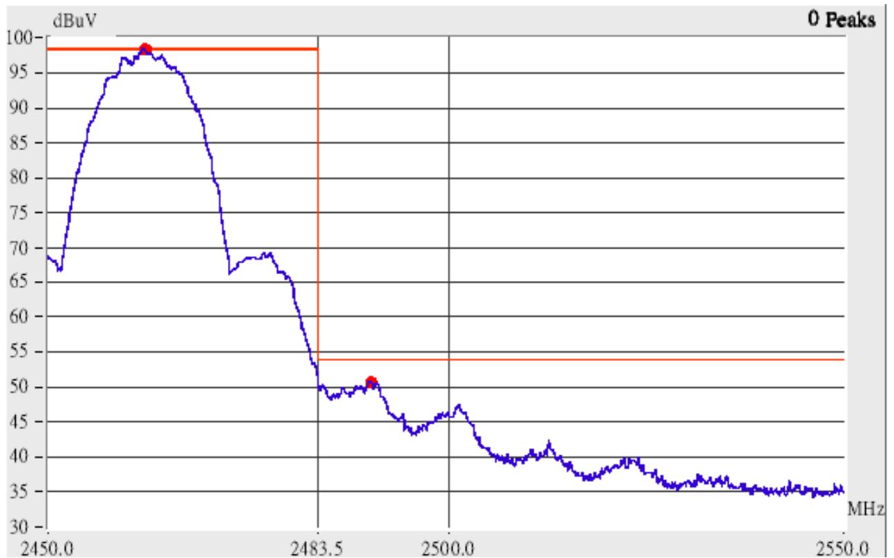
This is the hard copy of our bandedge measurement generated by our bandedge testing program. The pictures shown above is the bandedge of channel 1 and 11.
