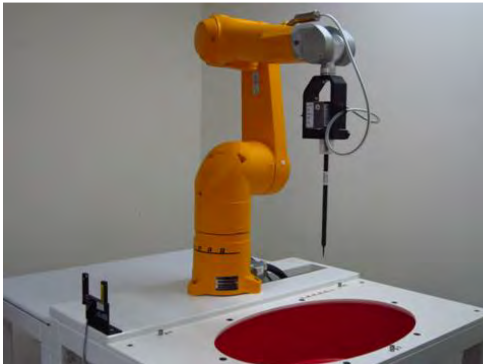
Fig.1 Photograph of the SAR measurement system
