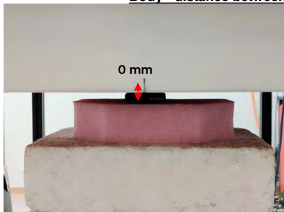
Fig.3 EUT Back side to flat phantom
