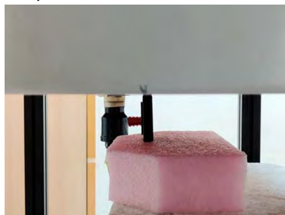
Fig.5 EUT Bottom side to flat phantom
