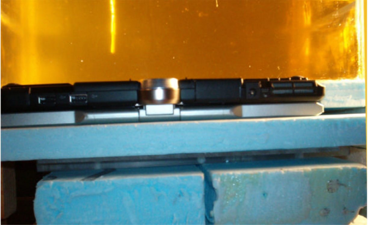
Fig. B. Side view photograph of the Toshiba PC for Configuration 1 of SAR testing. Since the SAR was too low to measure whether the display screen was folded onto the keyboard as for the closed cover condition or pointed outwards as for the tablet mode, this Configuration 1 determines the SAR distribution when the PC is placed on the laptop or for the tablet mode when the PC is held in the forearm as in Fig. 3-3 of the User's manual.
