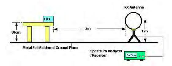
For Radiated Emissions: 30MHz~1GHz
