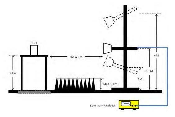
Above 10 GHz shall be extrapolated to the specified distance using an extrapolation factor of 20 dB/decade from 3m to 1m.
