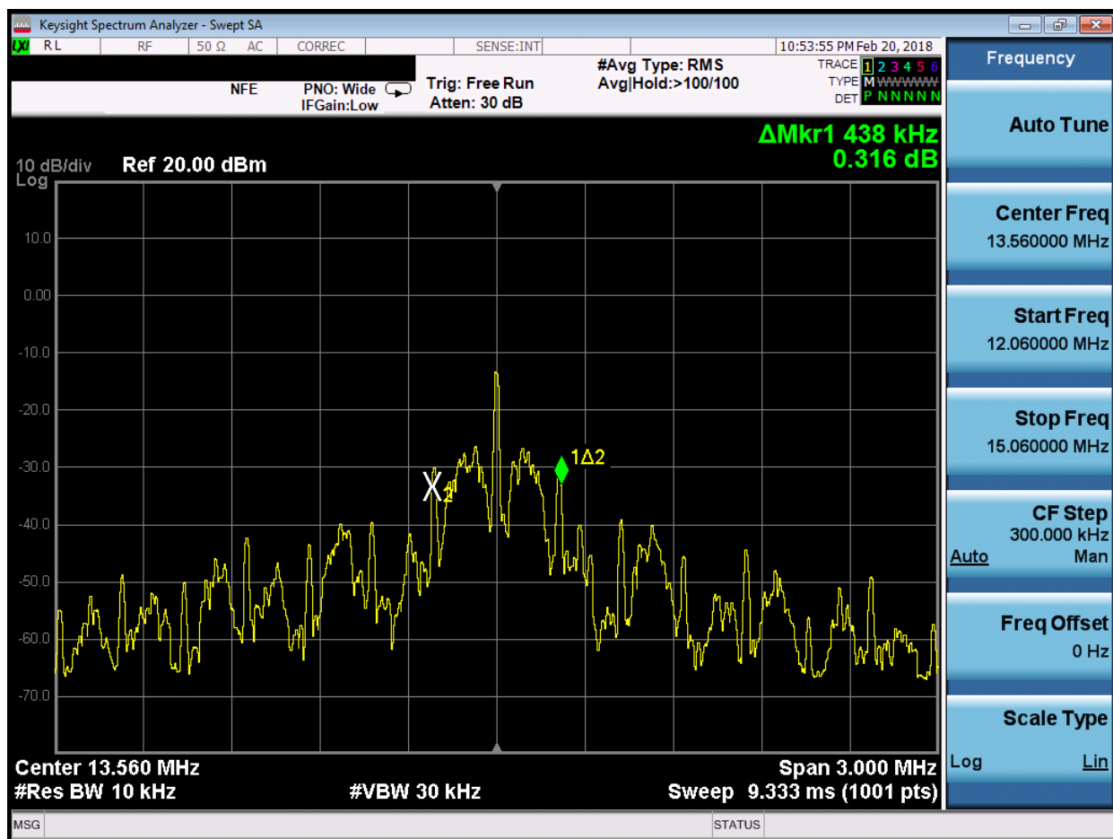
Figure 7-2. 20dB Bandwidth Plot
