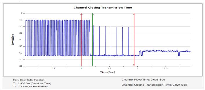
**Verdict**: Note: narrowing the sweep time as the good engineering process for the verification of transmission closing in 200ms
