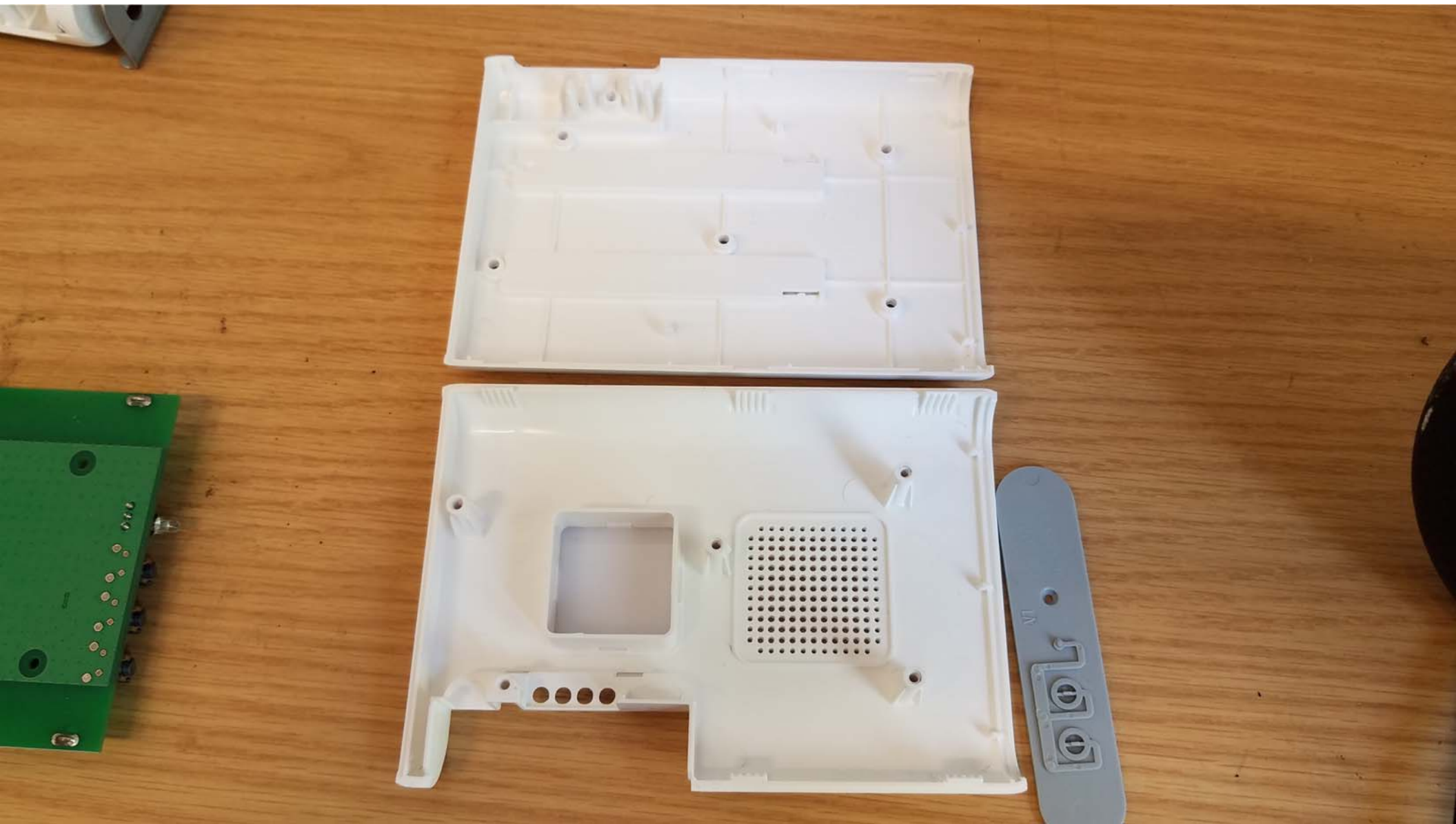
Inside View of the EUT - PCB's Removed
