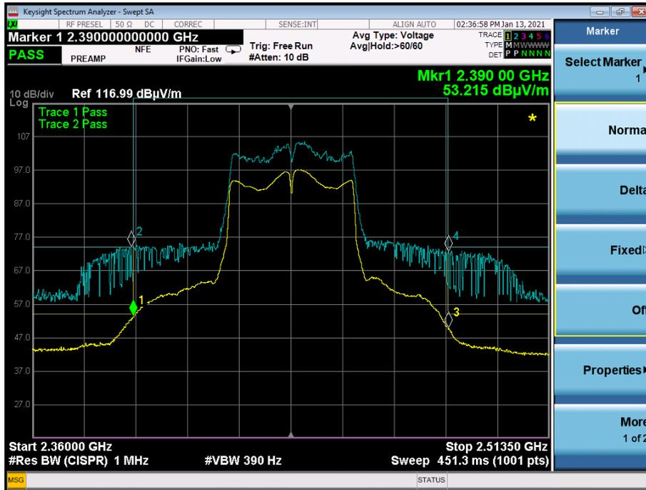
Graph 7: Radiated Lower Band Edge Plot – n 40 MHz Mode
