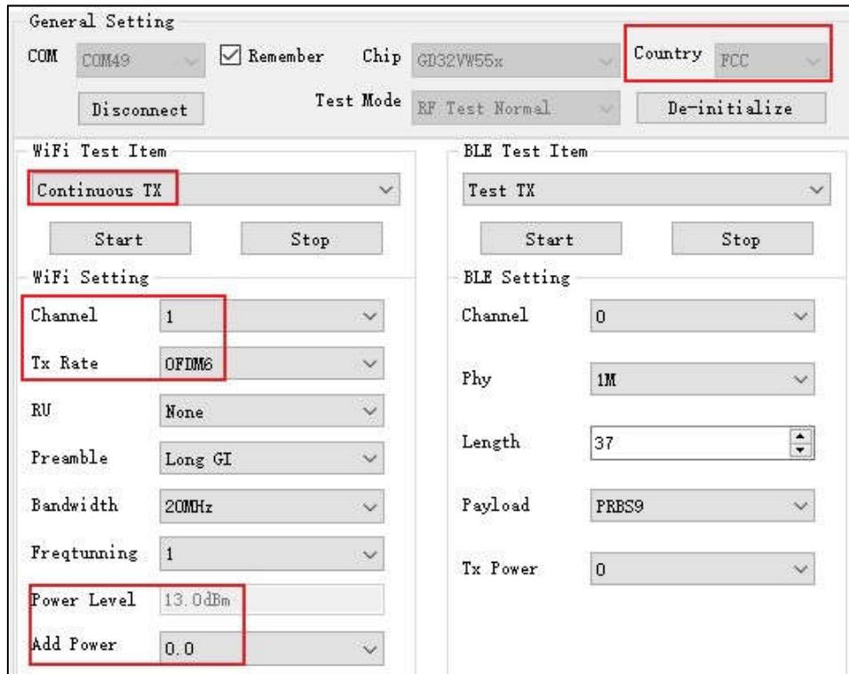
The screenshot displays the software's configuration window, divided into 'General Setting' and two test item sections: 'WiFi Test Item' and 'BLE Test Item'.
