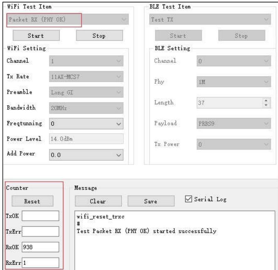
The screenshot displays the Packet RX (PHY OK) test configuration and results interface. It is divided into several sections:
