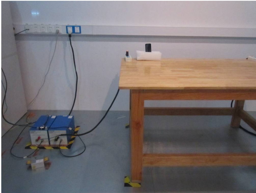
Conducted Emissions Test Setup Front View
