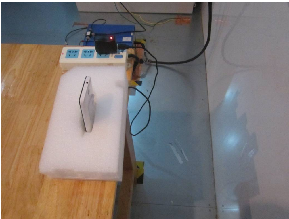
Conducted Emissions Test Setup Side View
