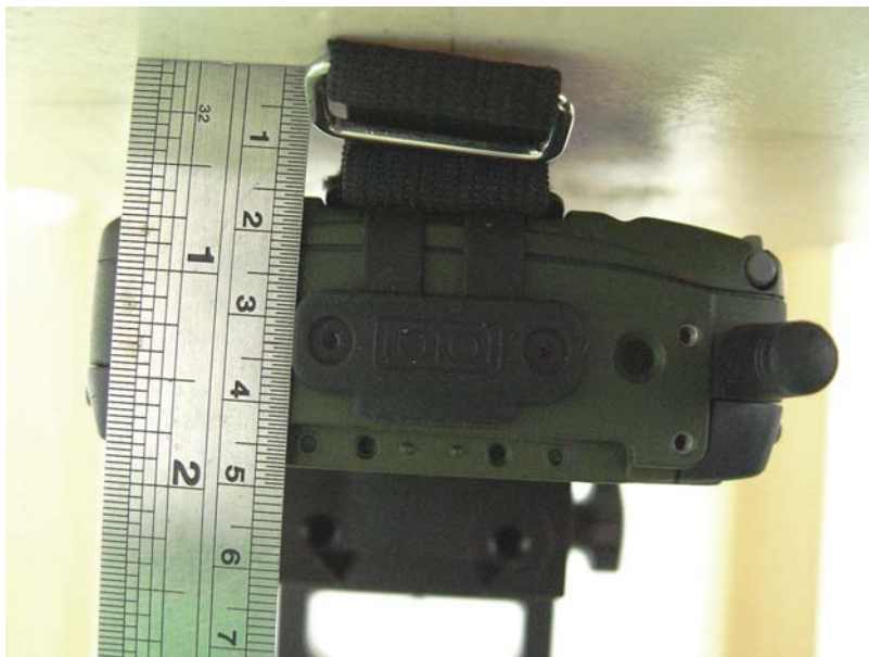
Fig. 9.8 Keypad Down with 1.5cm Gap
