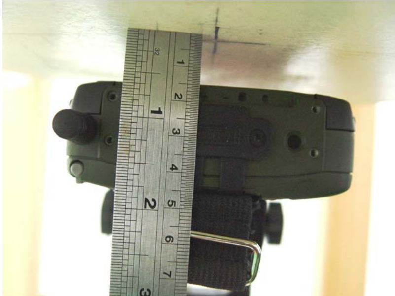
Fig. 9.7 Keypad Up with 1.5cm Gap
