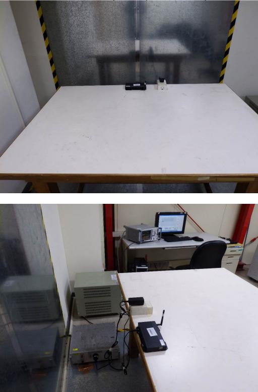
**Conducted Setup Photo (AC Power Line)**
