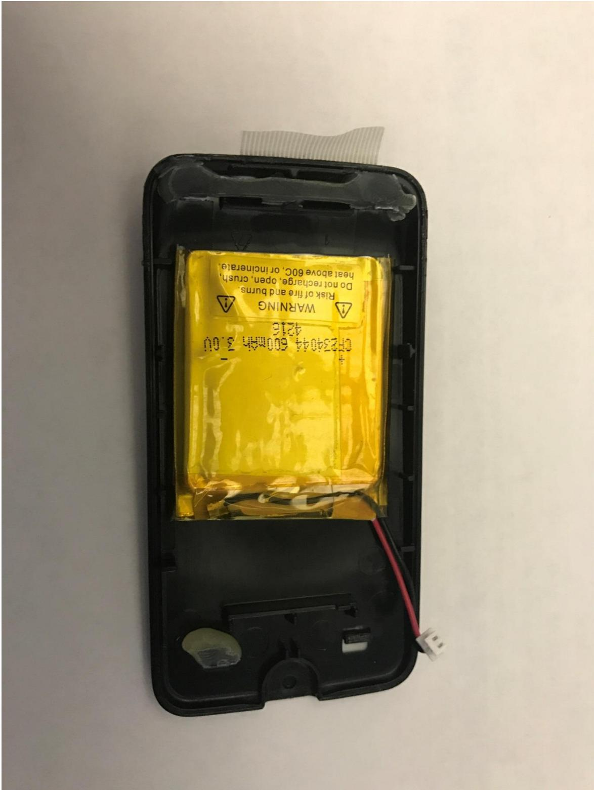
Back case, showing battery with PC board removed
