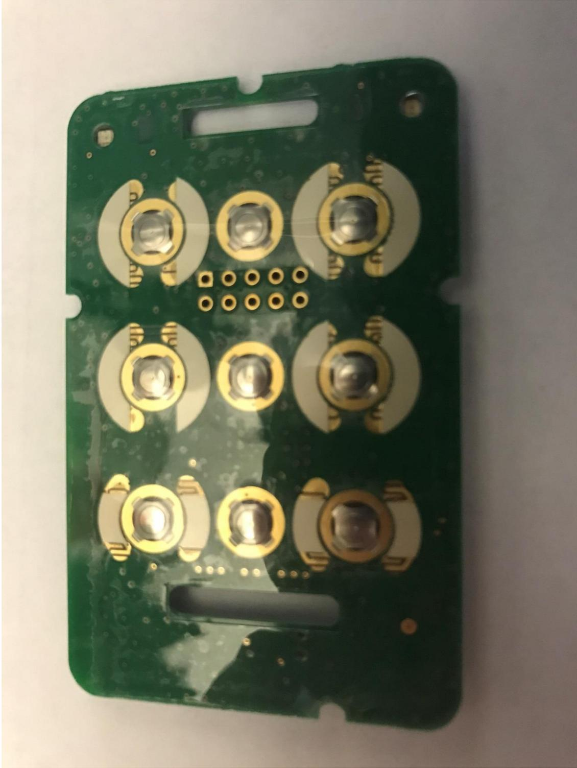
PC board front side, showing push button pads
