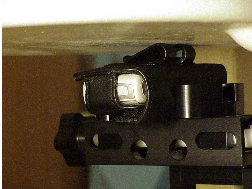
Device position against the body: Phone with belt holder under phantom
