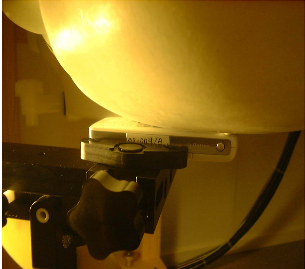
Device position against the head: Cheek (touch) phone position
