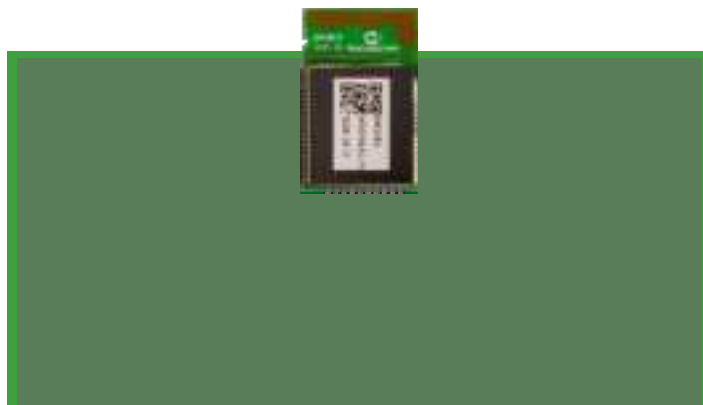
Figure 7-5. Recommended Module Placement
