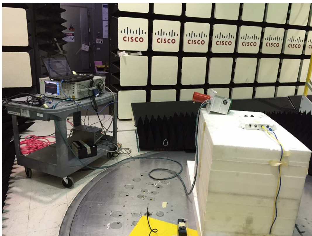
Title: Radiated Spurious Emissions Test Configuration 18 – 40GHz
